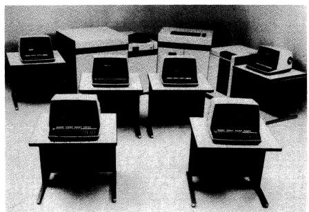
Features of the VS-100, top of Wang's VS family of virtual storage systems, include up to two megabytes of main memory, a 32K-byte cache memory, and 32-bit architecture. The VS-100 supports up to 4.6 billion bytes of disk storage and 128 workstations. The existing VS languages—COBOL, BASIC, RPG II, Assembler, and Procedure—are to be complemented by the addition of FORTRAN and PL/1. Prices for the VS-100 start at \$69,000.
