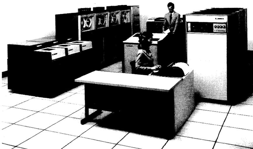
*The Xerox 560 computer system is designed to handle a broad range of applications including real-time, time-sharing, communications, and business data processing. It offers up to 262K 32-bit words of core storage with a 645-nanosecond cycle time.*
