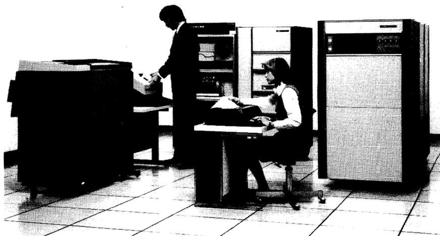
*The Xerox 550 is oriented toward engineering and scientific use in applications such as data acquisition and reduction, traffic control, factory automation, power utility control, and laboratory automation. The CP-R operating system allows concurrent processing of real-time, batch, and terminal programs.*
