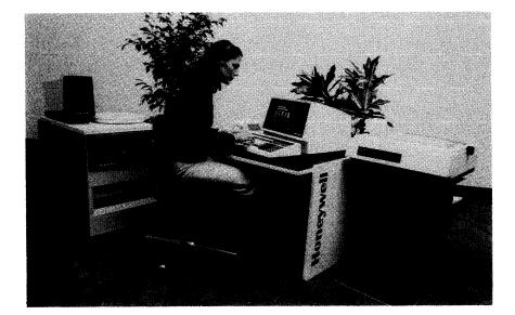
Honeywell's DPS 6 family of small computers includes the DPS 6/30, the 6/31, the 6/32 (pictured), the 6/34, and the 6/38 at the low end. Memory capacity for the systems ranges from 128K to 1024K bytes. Maximum disk storage capacity is from 10M to 1024M bytes. The systems accommodate a wide variety of printers ranging in speeds to 160 cps and 900 lpm. Purchase prices for the basic systems are \$19,500-\$30,000.
