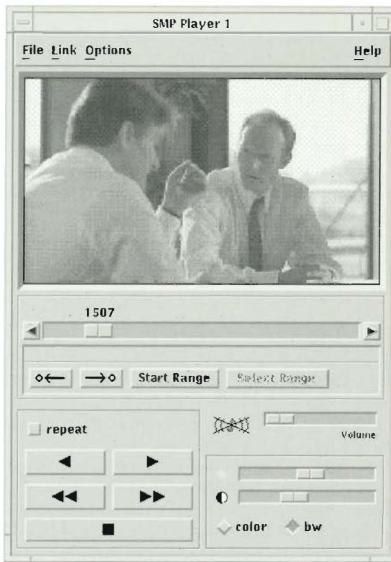
Figure 1 User Controls as Displayed on the Workstation Screen
