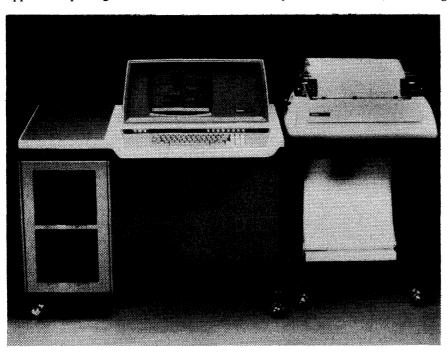
The Diablo 3200 system pictured here includes 32K bytes of RAM memory, four double density diskette units for 2.4 megabytes of storage and a Diablo matrix printer. The printer includes the print stand, forms tractor, and paper stand. The CRT console and diskette drives are housed in a workstation configuration.
