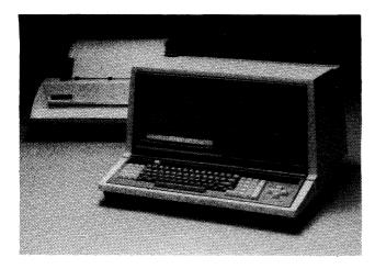
The Diablo 3000 system shown here with its associated Diablo matrix printer includes 32K bytes of RAM memory and two integral double density diskettes with a storage capacity of 1.2 megabytes in a compact tabletop configuration.
