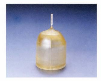
Fig. 13—As grown four-inch LN crystal under production at Fujitsu.
