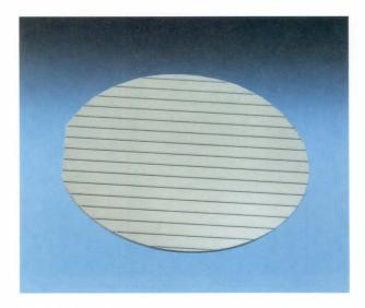
Fig. 35-Pattern-formed three-inch LN wafer (1018 4-MHz elements/wafer).
