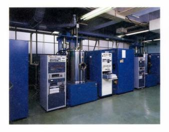
Fig. 12-Crystal growth stations at Fujitsu.
