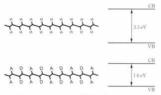
Fig. 19-Band gap control in PDA by donor and acceptor substitution.
