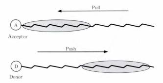
Fig. 12-Push- and pull-effects of donor (D) and acceptor (A). Donors push electrons and acceptors pull electrons when excited by light.
