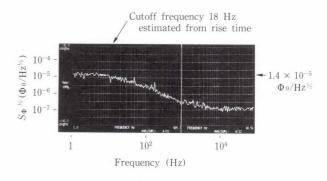
Fig. 36-Measured flux spectral density.
