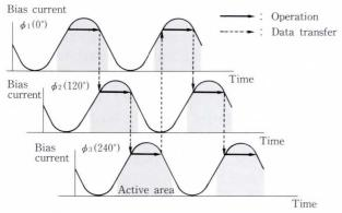
Fig. 22-Logic operation with three-phase sinusoidal power supply.
