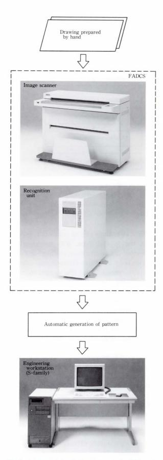
Fig. 6-Automated drawing input system for PC boards.
