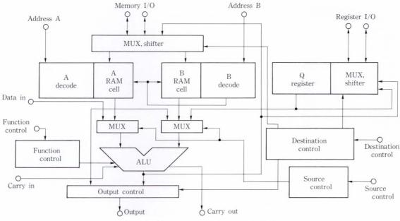
Fig. 32-Four-bit microprocessor diagram.
