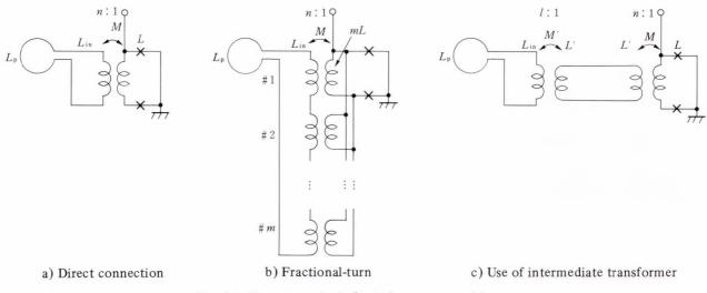
Fig. 21-Various methods for inductance matching.
