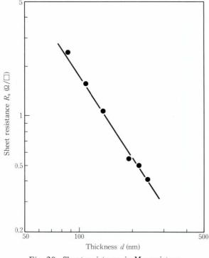
Fig. 20-Sheet resistance in Mo resistors.
