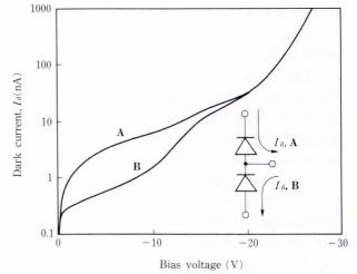
Fig. 9-Dark current versus bias voltage measured after flip-chip bonding.
