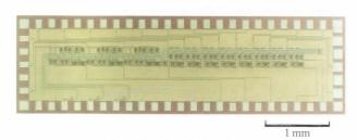
Fig. 53-Serial parallel converter.
