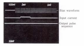
Fig. 9-Measured operation of the Josephson comparator.
