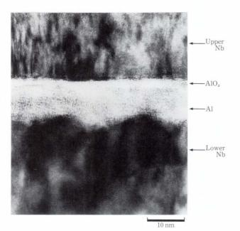
Fig. 46-Lattice image of Nb/AlO<sub>x</sub>/Nb junction structure.
