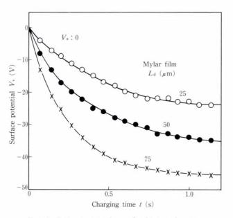
Fig. 4-Triboelectric charge for Mylar of various thickness.
