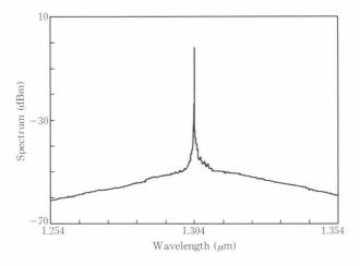
Fig. 22-OC-12 optical output spectrum.
