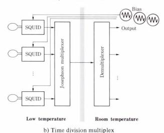
Fig. 4-Multichannel system with the single-chip SQUID.
