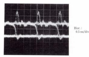
Fig. 23-OC-12 optical output waveform.
