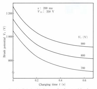
Fig. 13-Relationship between brush potential and charging time for selenium photoreceptor.
