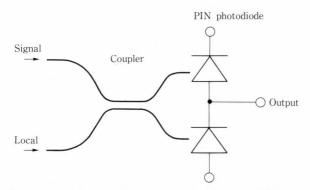
Fig. 1-Dual-detector balanced optical receiver (DBOR).
