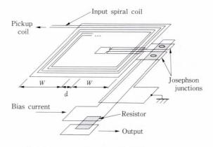
Fig. 18-Structure of the SQUID sensor.
