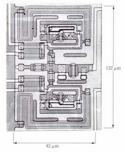
Fig. 15-Photomicrograph of 2OR-AND gate.
