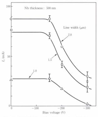
Fig. 43–Critical current  $I_c$  of bias-sputtered Nb films.
