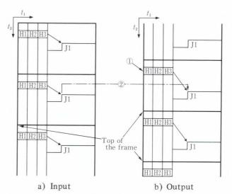
${\rm (D)}$  : Insert the pointer value indicating the timing of input J1.  ${\rm (2)}$  : Send data without delay after receiving it.
