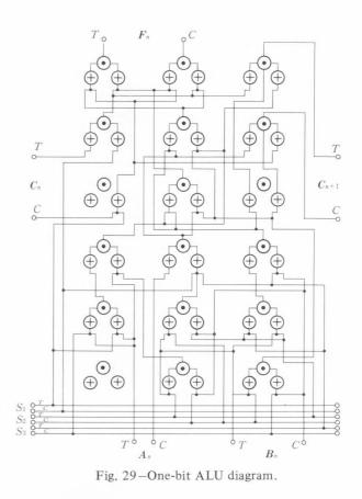
the 1-bit block shown in Fig. 29 are laid out for easy connection to the input terminals of the next block. This block can be used as a simple 1-bit slice ALU. When blocks are arranged serially, the input and output terminals are connected with the shortest possible wiring, resulting in a multiple-bit ALU using the ripple carry.
