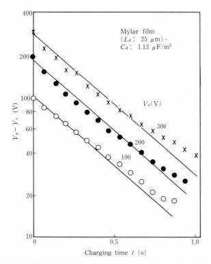
Fig. 5-Relationship between  $V_a - V_s$  and charging time for direct charge transfer.
