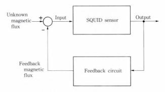
Fig. 2-Block diagram of the SQUID.
