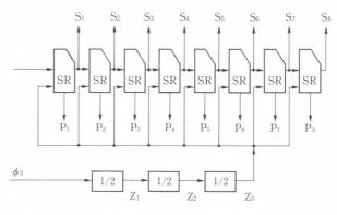
$S_n$ : Output from the 1-bit shift register in each bit.
