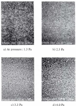
Fig. 4-SEM photographs of Nb films deposited at different Ar pressures. Film thickness is 600 nm.
