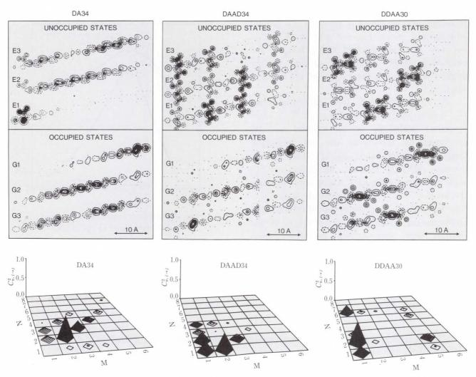
Fig. 14 – Contour diagrams of molecular orbitals near the Fermi surface in plane z-0.6 Å (0.06 nm) and  $C_{n,i \rightarrow j}^{2}$  for the first excited states. G denotes occupied orbitals and E unoccupied orbitals. G1 is HOMO and E1 is LUMO. *M* denotes the occupied molecular orbitals GM (M = 1, 2, ..., 6) and *N* unoccupied molecular orbitals EN (N = 1, 2, ..., 6). The height of the pyramid indicates  $C_n, GM \rightarrow EN^2$ .
