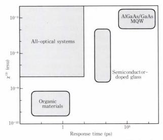
Fig. 8-Third-order nonlinear optical materials for alloptical devices.
