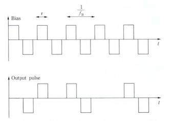
Fig. 11-The bias waveform and the output pulse of the Josephson comparator.
