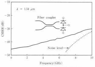
Fig. 11-Common-mode rejection ratio (CMRR) as a function of frequency.
