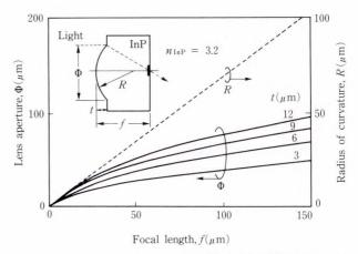
Fig. 4-Relationship between focal length (f), lens aperture  $(\Phi)$ , radius of curvature (R), and thickness (t) of the microlens.
