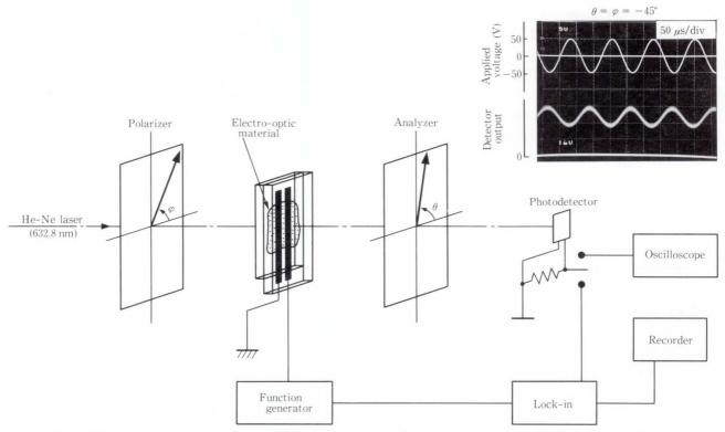
Fig. 6-Measurement system for AC modulation method and the typical light modulation signal for SPCD thin-film crystal.
