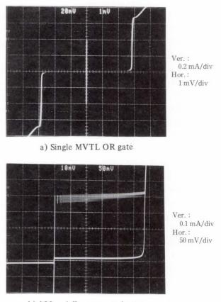
b) 100 serially connected gates
