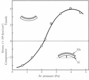
Fig. 5–Nb film stress versus Ar pressure during sputtering.
