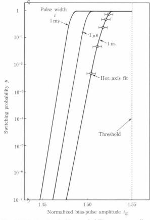
Fig. 34-Measured switching probability p vs normalized bias amplitude  $i_g$ .
