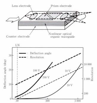
Electro-optic coefficient r (pm/V)
