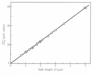
Fig. 27-Linearity of the tunneling current and the junction area.  $I_{\rm NN}$  is the tunneling current at 4 mV, and D is the side length of square junctions.
