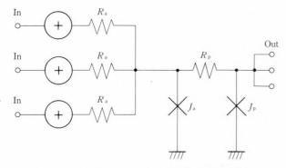
Fig. 16-Equivalent circuit of 2/3 majority gate.
