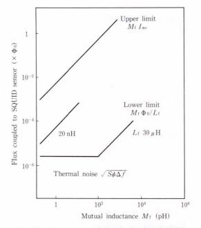
Fig. 27-Cover range of the single-chip SQUID.
