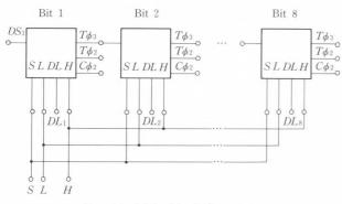
Fig. 25-Eight-bit shift register.
