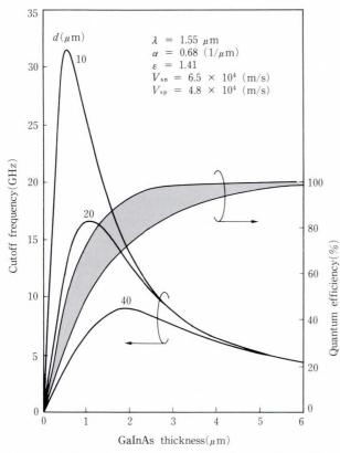
Fig. 3-Cutoff frequency and quantum efficiency as a function of GaInAs thickness. *d* is the PIN junction diameter,  $\alpha$  is the absorption coefficient of InGaAs at a 1.55- $\mu$ m wavelength,  $\epsilon$  is the dielectric constant of GaInAs,  $V_{sn}$  is the electron velocity, and  $V_{sp}$  is the hole velocity.
