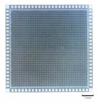
Fig. 34-Three-dimensional 10-Kgate array chip, 7.8 mm square. A 5 292 gates are integrated in both upper- and lower-level circuits.
