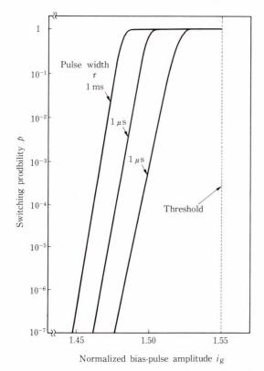
Fig. 13-Calculated switching probability vs normalized bias amplitude  $i_g$  (=  $I_g/I_0$ ).
