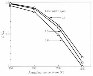
Fig. 18–Changes in  $I_c$  of wiring after annealing.
