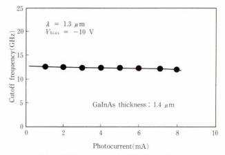
Fig. 12–Cutoff frequency as a function of photocurrent for optical input having a wavelength of 1.3  $\mu$ m.
