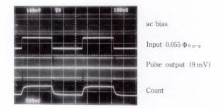
Fig. 32-Measured operation of the single-chip SQUID.
