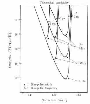
Fig. 17–Calculated square root of flux spectral density  $S_{\Phi}^{1/2}$  vs normalized bias amplitude  $i_g$ .
