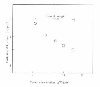
Fig. 11–Power-delay relationship of MVTL OR gate with a minimum junction diameter of  $1.2 \ \mu m^{3}$ .
