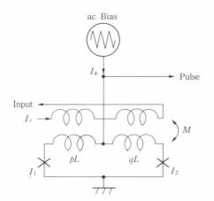
Fig. 5-Circuit of a Josephson comparator. It is a 2-junction interferometer without shunt resistor.
