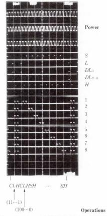
Fig. 27-Function tests of SHIFT, LOAD, HOLD, and CLEAR operations.
