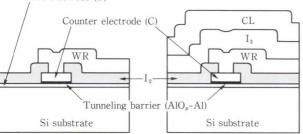
a) Without I<sub>3</sub> and CL layers b) With I, and CL layers Fig. 15-I-V characteristics and cross sections for junctions.
