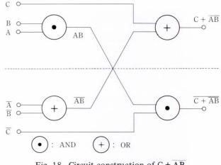
Fig. 18–Circuit construction of  $C + \overline{AB}$ .
