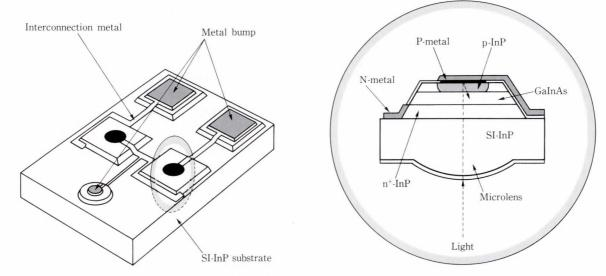
Fig. 2-Twin PIN photodiodes.
