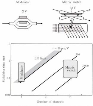
Fig. 4-Matrix optical switches and modulators, and correlation between the number of channels and switching time.
