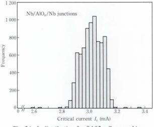
Fig.  $24-I_c$  distribution for 8 192 cells on a chip.
