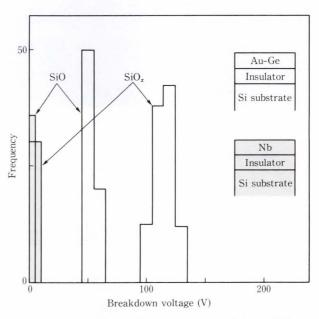
Fig. 13–Breakdown voltage in 300-nm SiO and  $SiO_x$  films.
