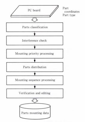
Fig. 8-Flow of data generation for mounting.
