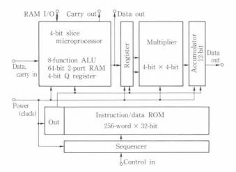
Fig. 35-Four-bit processor diagram.
