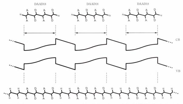
Fig. 20-Multiple quantum well formation in PDA. Wells can be regarded as DAAD18 molecules inserted in a PDA chain.
