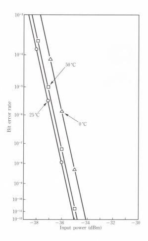
Fig. 24–OC-12 LR (1.31 µm) bit error rate characteristics.
