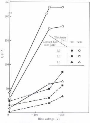
Fig. 44–Critical current  $I_c$  of contacts versus bias voltage during Nb sputtering.
