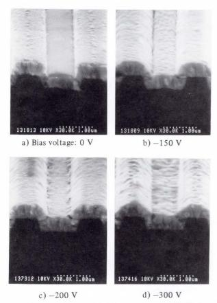
Fig. 42-Cross-sectional SEM photographs of Nb deposited on  $SiO_2$  steps. Nb and  $SiO_2$  are 500 nm thick.
