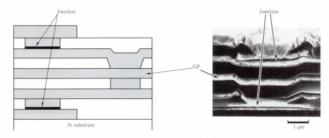
Fig. 35-SEM photograph of a vertically stacked gate array.
