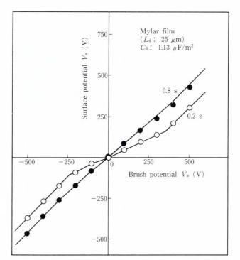
Fig. 8-Relationship between surface potential and brush potential.
