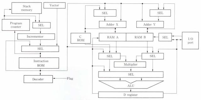
Fig. 37-Eight-bit DSP diagram.
