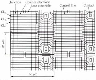
Fig. 21-Cell layout for the 8K-bit memory cell array chip. The unit cell is indicated by a bold rectangle.
