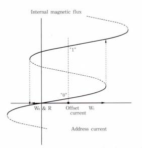
b) Memory operation on internal flux vs external flux curve (W<sub>1</sub> denotes write 1, and W<sub>0</sub> & R denotes write 0 and read)
