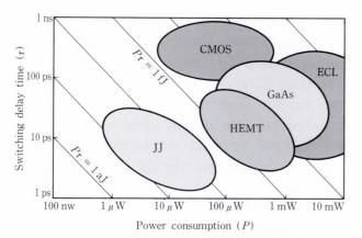
Fig. 1-Relationship of switching time and power consumption for different high-speed logic gates.
