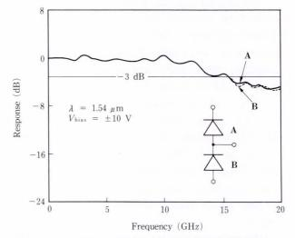
Fig. 10-Frequency response characteristics monitored for an optical input signal having a wavelength of  $1.54 \ \mu m$ .
