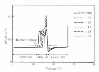
Fig. 41–Anodization profiles of Nb/AlO<sub>x</sub>/Nb junctions with five different Al thicknesses. The upper and lower Nb are 30 nm and 15 nm thick.
