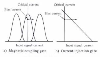
Fig. 3-Threshold characteristics.
