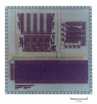
Fig. 36-Four-bit processor.
