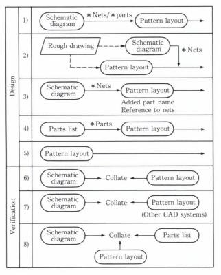
Fig. 2-Flexible design flow and some collations.
