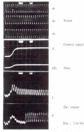
Fig. 28-Measured SHIFT operation with 2.3 GHz (430 ps) clock.
