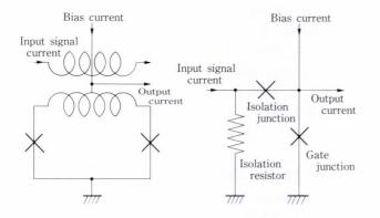
a) Magnetic-coupling gate b) Current-injection gate
