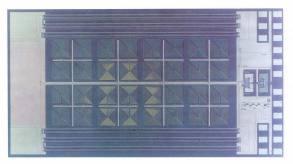
Fig. 30-Photograph of the improved single-chip SQUID.
