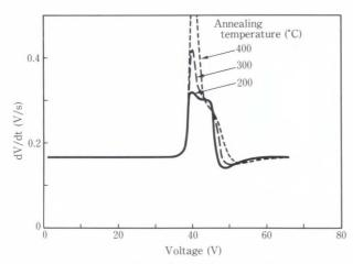
Fig. 39–Anodization profiles of Nb/AlO<sub>x</sub>/Nb junctions annealed for 30 min.
