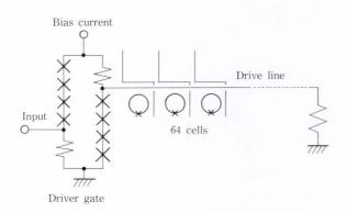
Fig. 45-Equivalent circuit of driver gate. A cell drive line is also shown. The critical current of all junctions is 4.2 mA. The resistance for each of the two resistors is  $1.5 \Omega$ .
