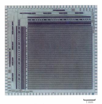
Fig. 46-4 K-bit memory circuit.
