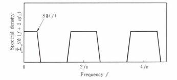
Fig. 16-Spectral density with aliasing effect.
