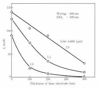
Fig.  $17-I_c$  of wirings versus the thickness of underlaying Nb base electrode.
