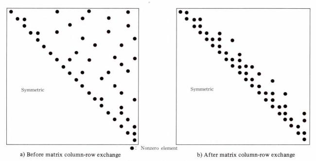
Fig. 4-Matrix column-row exchange.
