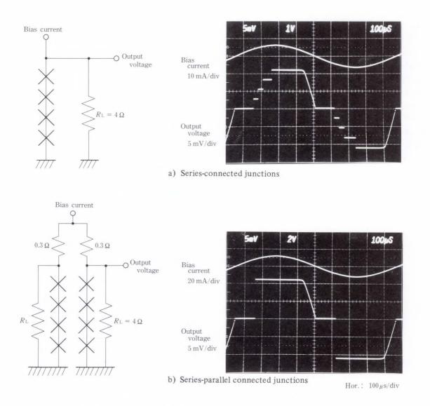
Fig. 48-Voltage waveforms across junctions driven by sinusoidal current.
