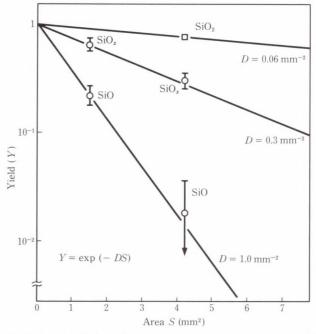
Fig. 23–Yield of the insulation checks versus the area of the insulators.
