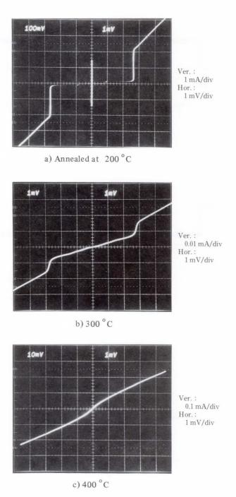
Fig. 40-I-V characteristics of junctions.
