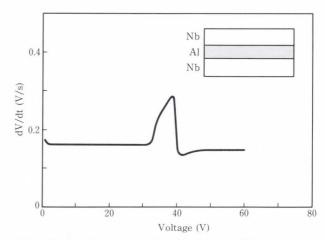
Fig. 38-Anodization profile for a Nb/Al/Nb structure.
