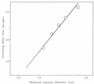
Fig. 12-Relationship between fastest gate delay and minimum junction diameter of MVTL OR gate.
