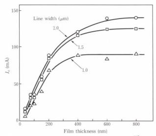
Fig. 16–Critical current  $I_c$  of Nb wiring lines<sup>77)</sup>.
