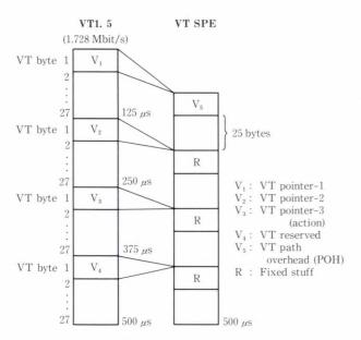
Fig. 8-VT1.5 superframe structure.
