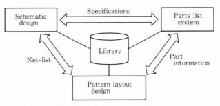
Fig. 5-System linked by parts list system.
