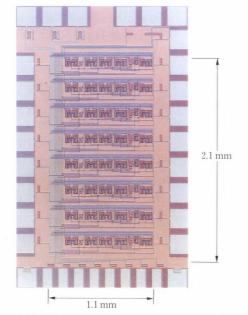
Fig. 26-Fabricated 8-bit shift register chip.
