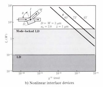
Fig. 7-Correlations between  $\chi^{(3)}$  and the light power required for device operation.
