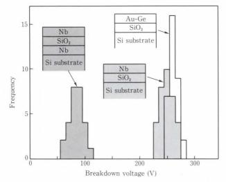
Fig. 14-Breakdown voltage in 300-nm sputtered SiO<sub>2</sub> films.
