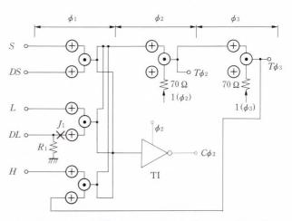
Fig. 24–One-bit shift register circuit. Input resistor  $R_{in}$  for the OR gate and TI and supply resistor  $R_s$  for the OR gates are omitted.
