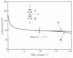
Fig. 8-Photodiode capacitance versus bias voltage measured before flip-chip bonding.
