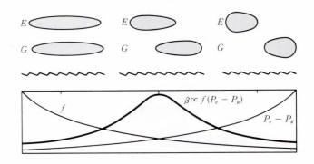
Fig. 11-Relationship between second-order optical nonlinearity and wave function separation.
