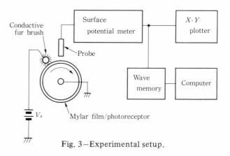
to +700 V is applied to the brush. The probe of a surface potential meter is positioned over the drum. The probe output can be displayed visually on an X-Y plotter, or it can be digitized and stored for analysis.
