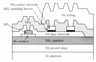
Fig. 2–Integrated circuits with Nb/AlO<sub>x</sub>/Nb Josephson junctions.
