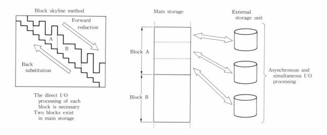
Fig. 7-Block skyline method and parallel I/O method.
