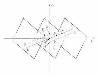
Fig. 25-The operating trajectory on the threshold curve of the write gate.
