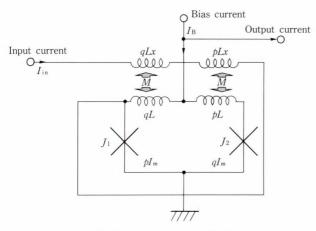
a) Basic structure for the MVTL OR gate, whose input current both couples to the interferometer magnetically and it is injected.
