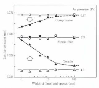
Fig. 29-Changes in the Nb lattice constant during patterning (Hollow symbols: before patterning, solid symbols; after patterning).
