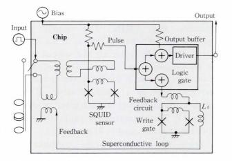
Fig. 29-Circuit of the improved single-chip SQUID.
