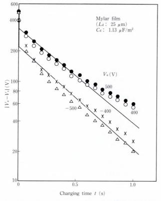
Fig. 7-Relationship between  $V_a - V_s$  and charging time for gas discharge process.
