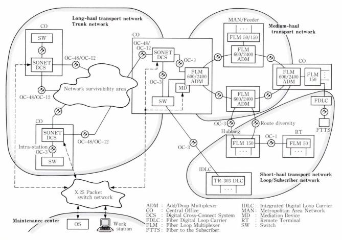
Fig. 1-System application for SONET.
