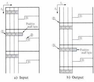
D : Receiving pointer value with increment bits inverted. D : Detect the phase difference between the input J1 and
