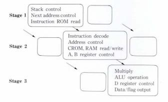
Fig. 38-DSP processing sequence.
