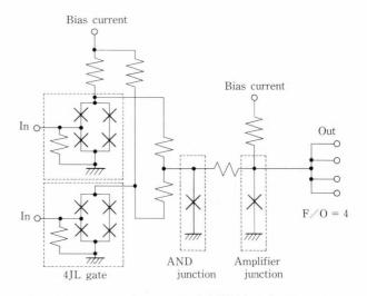
Fig. 43-Equivalent circuit of AND gate for decoder.
