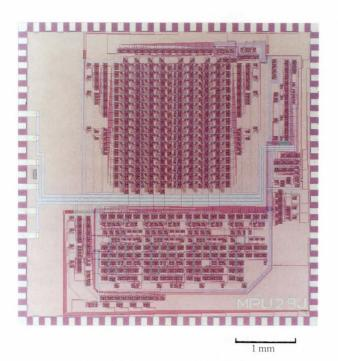
Fig. 33-Four-bit microprocessor.
