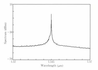
Fig. 19-OC-3 optical output spectrum.
