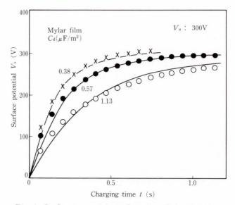
Fig. 6-Surface potential as a function of charging time.
