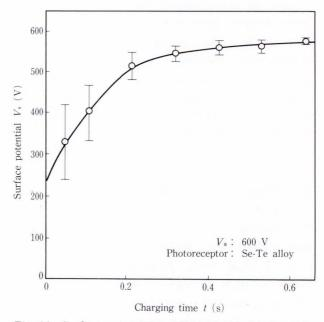
Fig. 11-Surface potential as a function of charging time for selenium photoreceptor.
