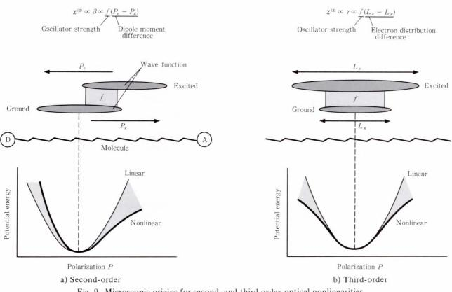
Fig. 9-Microscopic origins for second- and third-order optical nonlinearities.
