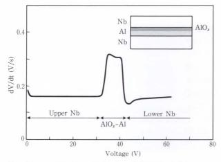
Fig. 37-Anodization profile for a Nb/AlO<sub>x</sub>/Nb junction. The upper Nb and Al layers are 30 nm and 7 nm thick.
