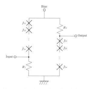
Fig. 49-Equivalent circuit for the high-voltage gate interfacing Josephson junctions and semiconductors.
