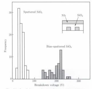
Fig. 30-Breakdown voltages of sputtered and bias sputtered SiO<sub>2</sub> films deposited on patterned Nb films.
