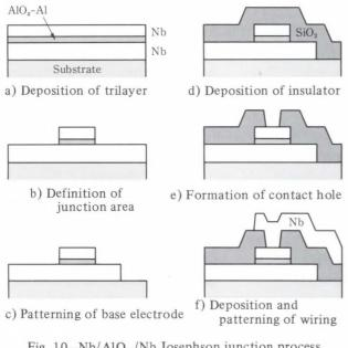
Fig. 10–Nb/AlO<sub>x</sub>/Nb Josephson junction process sequence.
