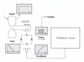
Fig. 22-Operation of the digital SQUID.
