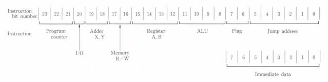
Fig. 39-24-bit instruction code format and immediate data format.
