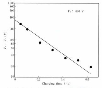
Fig. 12-Relationship between  $V_a - V_s$  and charging time for selenium photoreceptor.
