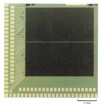
Fig. 22-Microphotograph of the fabricated 8K-bit memory cell array.
