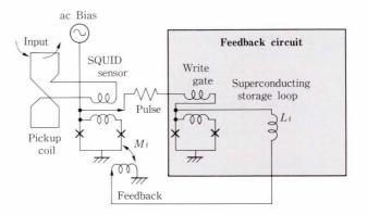
Fig. 26-Circuit of the single-chip SQUID.
