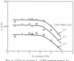
Fig. 6–Critical current  $I_c$  of Nb wirings versus Ar pressure.
