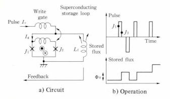
Fig. 24-Superconducting feedback circuit.
