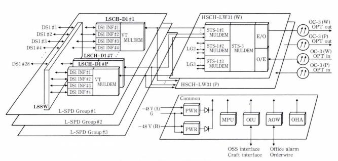
Fig. 6-Block diagram of FLM 150.
