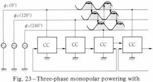
Fig. 23-Three-phase monopolar powering with sinusoidal waves.
