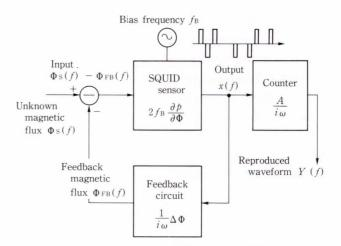
Fig. 23-Block diagram of the digital SQUID for small input flux. Only the frequency componentbelow the bias frequency  $f_{\rm B}$  is considered.
