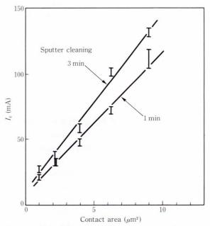
Fig. 19–Critical current  $I_c$  in contacts formed between Nb electrodes<sup>77)</sup>.
