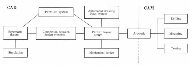
Fig. 1-Structure of PC board CIM system.
