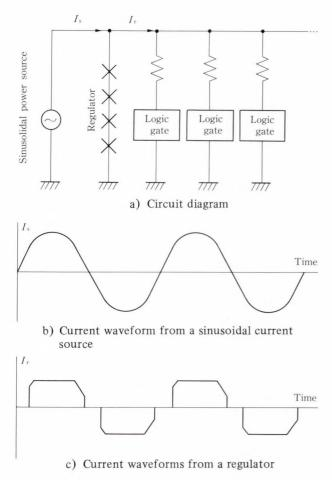
Fig. 19-Alternate current powering with single-phase power supply.
