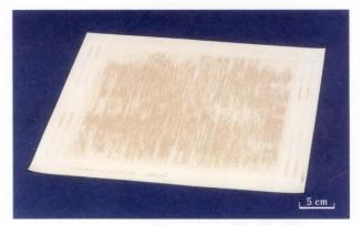
Fig. 10-Green sheet with copper pattern.
