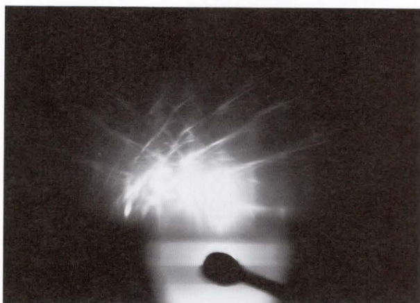
Fig. 3—RHEED pattern from a photoepitaxially grown layer at 630 °C. The photoepitaxial layer thickness is 200 nm.
