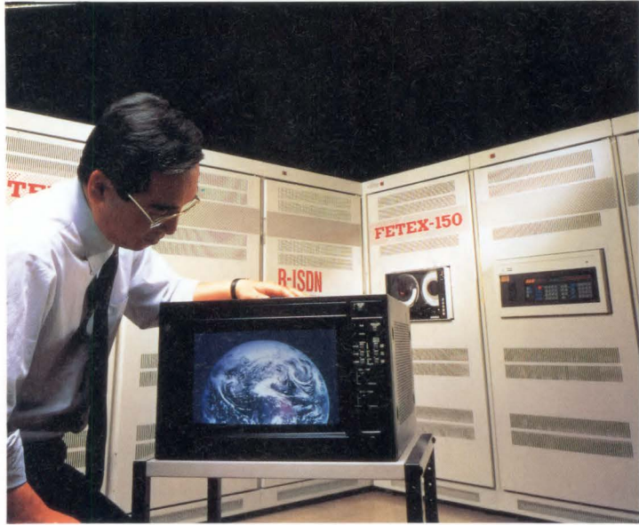
FETEX-150 B-ISDN Switching System
