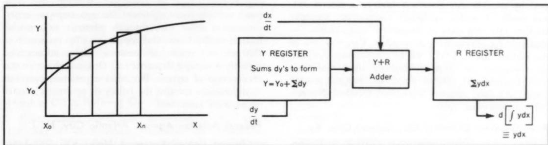
Figure 10. Block diagram of digital integrator used in the digital differential analyzer and approximation of the integral by summation. (Courtesy, Litton Industries.)
