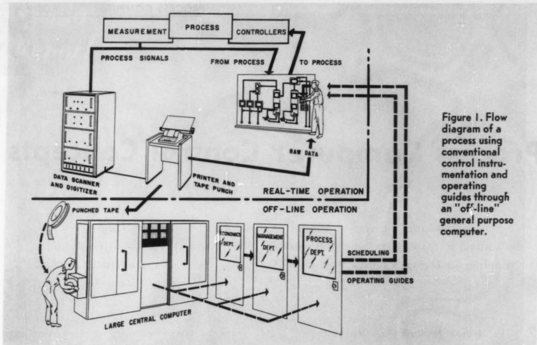
Figure 1. Flow diagram of a process using conventional control instrumentation and operating guides through an "off-line" general purpose computer.
