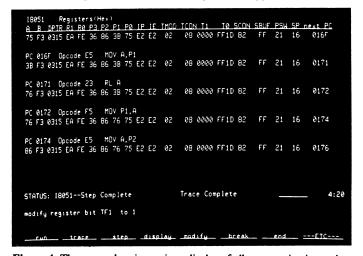
Figure 4. The comprehensive register display of allows examination and modification of all internal 8051 registers. Registers with specific control bits are supported by name on the HP 64000 softkeys for convenient modification.
