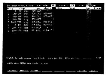
Figure 1. Flexible mapping permits memory resources to be allocated in 256-byte blocks. Separate mapping of Program and External data memory into the prototype or emulation subsystem provides additional resolution.
