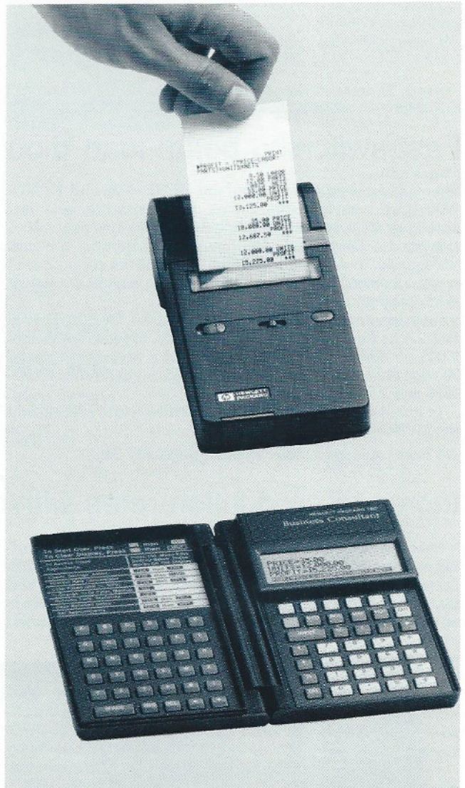
The portable HP 82240A Infrared Printer communicates via an infrared light beam.
