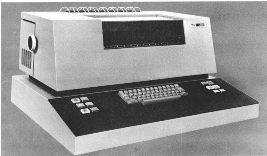
Figure 3. IBM 3215 Console Printer-Keyboard Model 1
