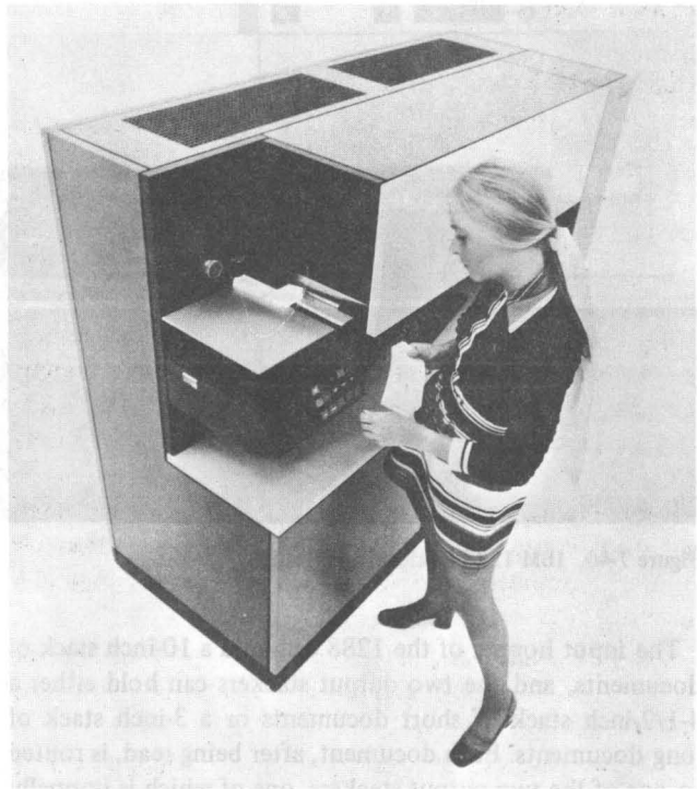
Figure 7-42. IBM 3886 Optical Character Reader
