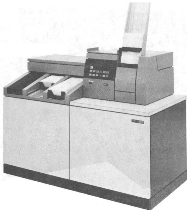
Figure 7-62. IBM 3504 or 3505 Card Reader
