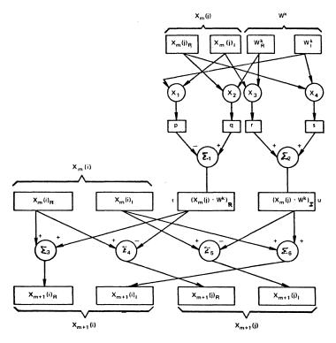
Figure 5. Data flow graph for FFT butterfly
