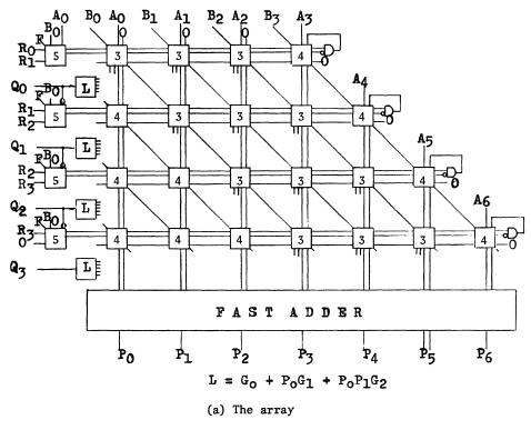
Figure 2 (cont'd.). MD2 - Multiplier/Divider array using Booth and Nonrestoring algorithms and Carry-save along with Carry lookahead, for n=4.
