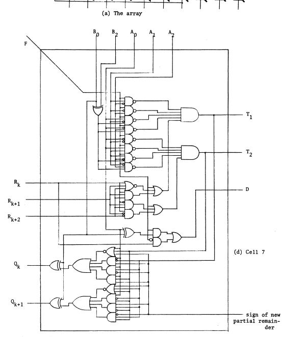
Figure 3 (cont'd.). MD3 - Multiplier/Divider array using multiplier bit pair grouping and 2-bit quotient generation, for n=5.
