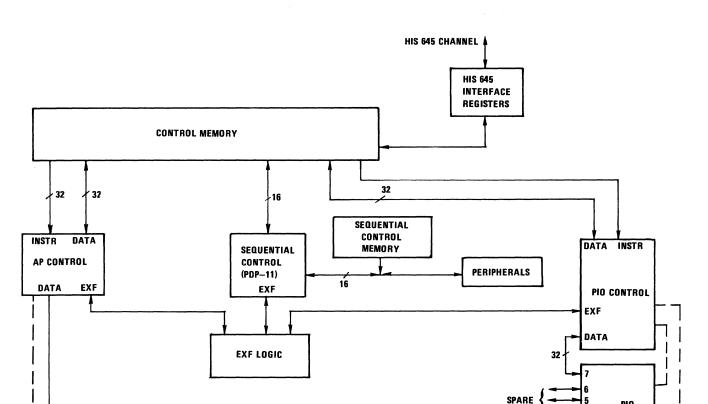
Figure 5. STARAN/RADCAP Block Diagram
