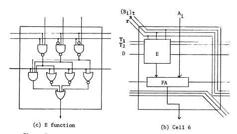
Figure 3. MD3 - Multipler/Divider array using multiplier bit pairing and 2-bit quotient generation, for n=5.
