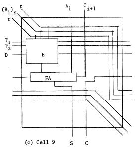
Figure 4. MD4 - Multiplier/Divider array using multiplier bit pairing and 2-bit quotient generation with carry-save and carry lookahead technique, for n=6.
