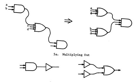
5b. DeMorgan's Theorem Figure 5. Depth Reduction for Combinatorial Nets
