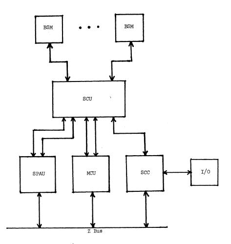
Figure 1. AN/UYK-17 System Block Diagram
