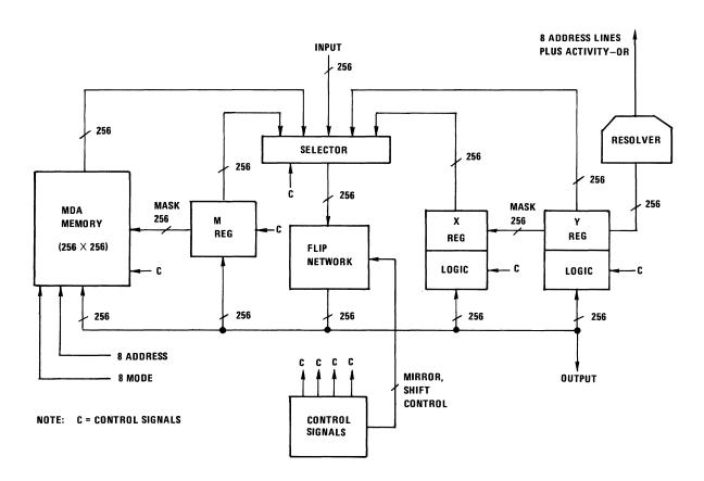
Figure 4. STARAN Array Module
