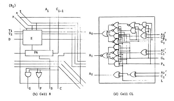
Figure 4 (cont'd.). MD4 - Multiplier/Divider array using multiplier bit pairing and 2-bit quotient generation with carry-save and carry lookahead technique, for n=6.
