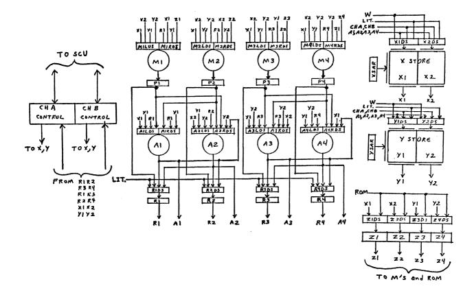
Figure 4. SPAU arithmetic section
