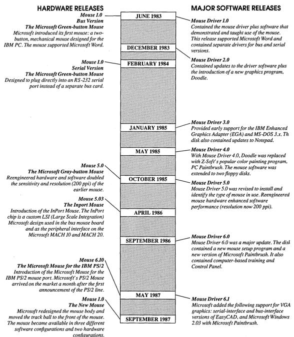
Figure 1-7. Major hardware and software releases of the Microsoft Mouse.
