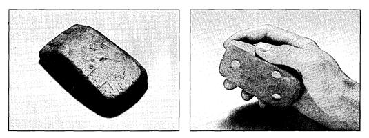
Figure 1-2. The clay model for the original Microsoft Mouse.
