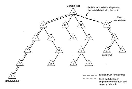
**Figure 13-1.** The trust relationship established between the forest root and the additional tree's uppermost domain. Also illustrated is the way in which the forest root treats the trust relationship.
