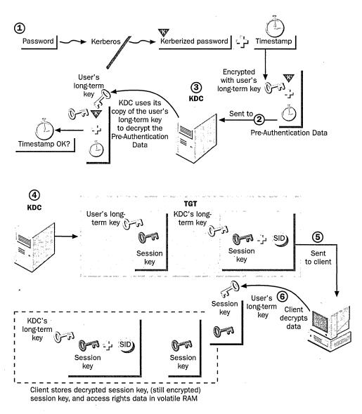
Figure 8-2. Kerberos authentication with AS Exchange.
