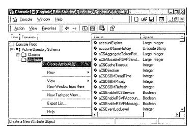
Figure 9-72. Adding a new attribute object to the schema.
