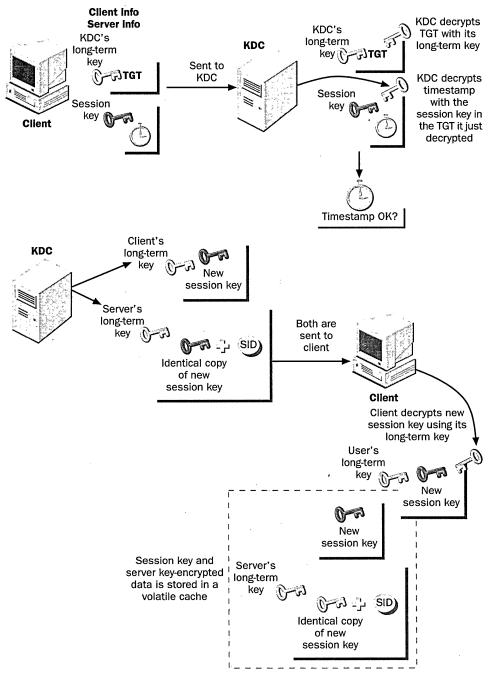
Figure 8-3. KDC interaction with TGS Exchange.
