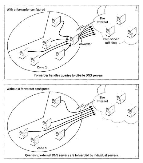
Figure 6-3. Using forwarders to minimize the number of DNS servers communicating with the outside world.
