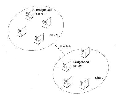
**Figure 9-99.** Two sites in an Active Directory deployment, with multiple domain controllers and one bridgebead server in each site.
