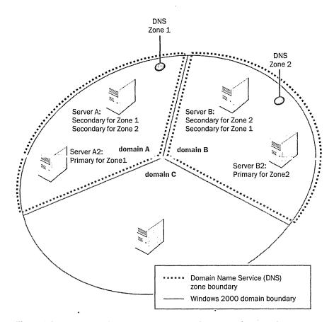
Figure 6-2. Using a single DNS server as a secondary server for more than one zone.
