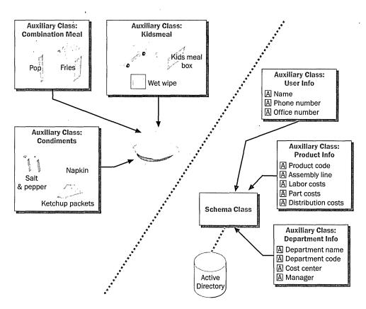
Figure 10-1. How auxiliary classes work in Active Directory services and in the drivethrough.
