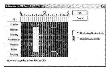
**Figure 9-57.** Specifying time blocks to keep replication traffic from taking up site link bandwidth during a specified time period.
