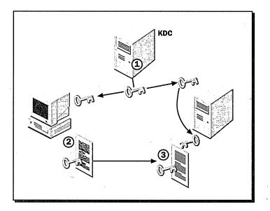
(1) KDC provides a unique key to a client and server that want to communicate in a secure way.
