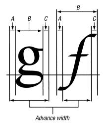
An application can use the **GetCharABCWidths** function to retrieve the ABC spacing for characters in a TrueType font.
