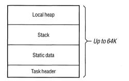
The size of the stack is always fixed for a given application. You specify the size, in bytes, of the stack by using the **STACKSIZE** statement in your application's module-definition (.DEF) file. Windows enforces a minimum stack size of 5K. You should experiment with your application to determine an optimum stack size, although keep in mind that the results of a stack overflow are unpredictable.
