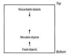
As Windows adds new objects to an application's local heap, movable objects may move as Windows compacts the heap. Also, Windows may discard some objects to make room for new ones. Windows never moves fixed objects when they are allocated in a local heap.
