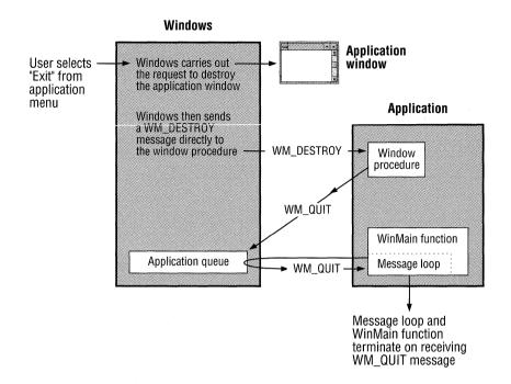
When the message loop retrieves the WM\_QUIT message, the loop terminates and the main function exits.
