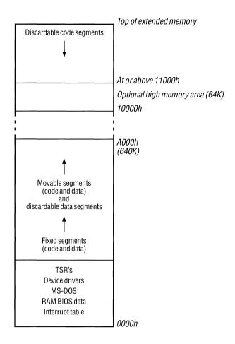
As with other memory configurations, Windows allocates discardable code segments from the top of the heap, fixed segments from the bottom of the heap, and movable code and data segments above fixed segments.
