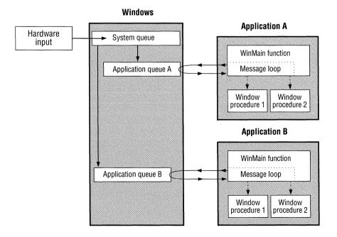
Windows can receive and distribute input messages for several applications at the same time. As shown in the following figure, Windows collects input messages in its system queue and then copies each message to the appropriate application queue. Again, the message loop in each application retrieves messages and dispatches them, through Windows, to each application's appropriate window procedure.
