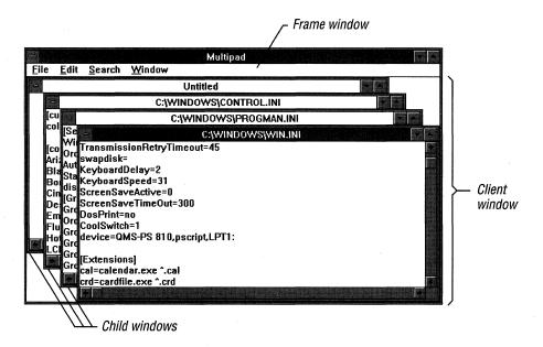
In general, an application controls the MDI interface by passing messages up and down the hierarchy of MDI windows. The MDI client window, which Windows controls, carries out many operations on behalf of the application.
