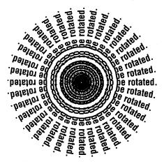
The **lfOrientation** member of the **LOGFONT** structure is ignored by GDI, which currently, assumes that the values for **lfEscapement** and **lfOrientation** are identical.
