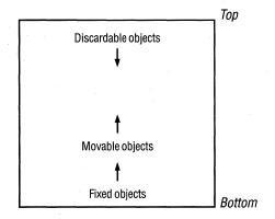
As Windows adds new objects to an application's local heap, movable objects may move as Windows compacts the heap. Also, Windows may discard some objects to make room for new ones. Windows never moves fixed objects when they are allocated in a local heap.
