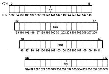
Figure 6-3. Runs of a Compressed Sparse File
