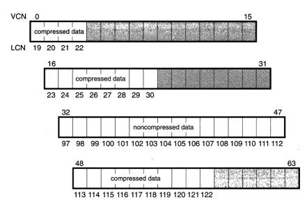
Figure 6-5. Data Runs of a Compressed File
