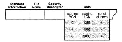
Figure 6-2. MFT Record for a Noncompressed File
