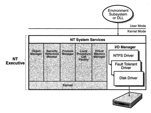
Figure 2-1. Components of the Windows NT I/O System
