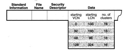
Figure 6-4. MFT Record for a Compressed Sparse File
