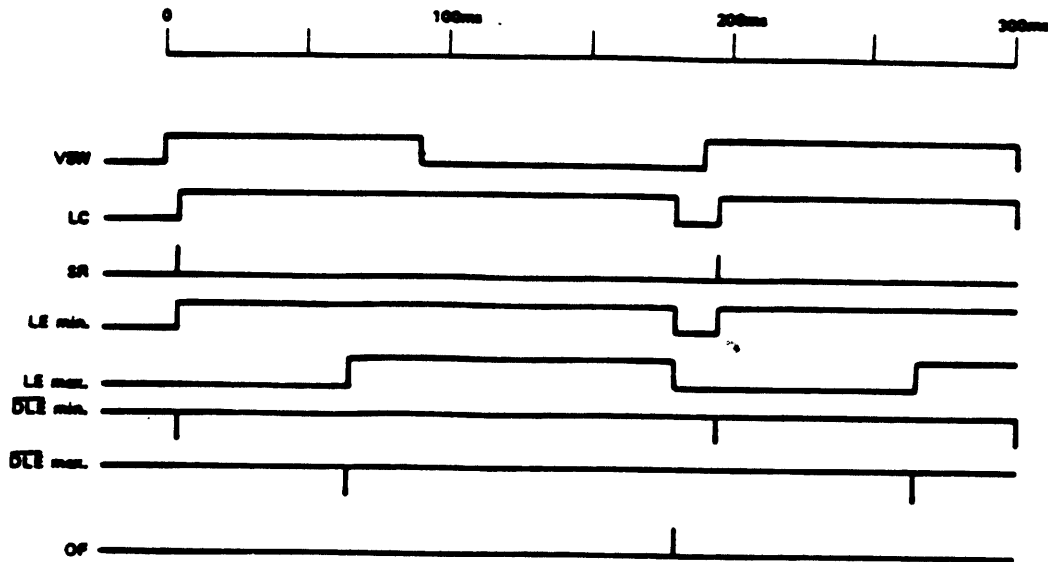
Figure 2. Timing diagram for Polaroid controller board signals.
