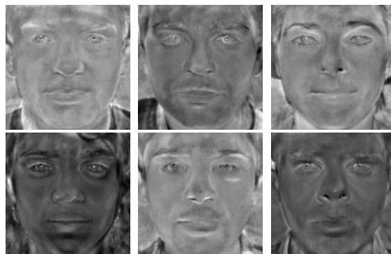
Figure 6-7: Example textures processed by the pseudoinverse T^\dagger = (T^t T)^{-1} T^t . When using the original set of image textures as a basis, texture analysis is performed by projection onto these images.
