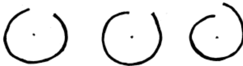
Figure 3-21. A series of boundaries to be closed. The points required to join the leftmost boundary would all have small deviations and the join seems good. The points required to join the rightmost boundary would have abysmal deviations and the join seems bad. The middle boundary is intermediate.
