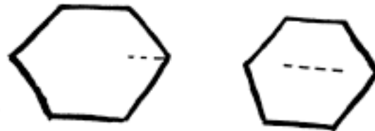
Figure 3-27. A hexagon. The Smoothed Local Symmetries in the corners (left) and between opposite sides (right) are salient, despite the fact that a hexagon is an LRS region.
