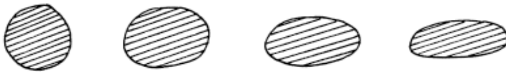
Figure 3-18. A set of ovals that are increasingly flattened. As the ovals are flattened, the average angular deviation increases and the region becomes less good as a round region.
