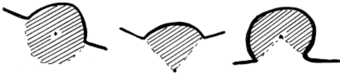
Figure 3-14. The left-hand example shows the region bounded by a partial round boundary plus a smooth join of its ends. The middle and right-hand figures show the regions obtained using the union of the radii of a partial round region. Neither of these definitions matches the perceived area of a partial round region.
