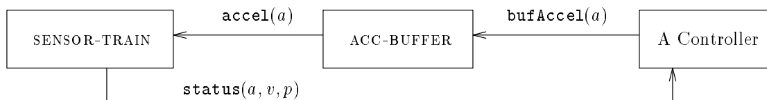
Figure 6-1 Overview of Feedback with Delay Deceleration Model
