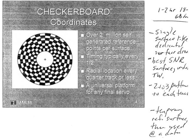
"CHECKERBOARD" Technology is a patented and <u>industry proven</u> process that uses the drive itself to write a very precise set of universal references that are in turn used for controlling the writing of any final drive servo information. This technology has been licensed to, and used in production by the largest manufacturer of disk drives in the world.
