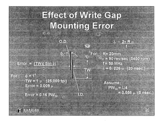
The task of matching adjacent track servo information and shingle writing has become much more difficult as servo frequencies and thus bit densities have continued to increase. With servo frequencies equal to or exceeding 50 MHz and the  $PW_{50}$  less than 5 nanoseconds, it becomes necessary to maintain timing to sub-nanosecond tolerances.
