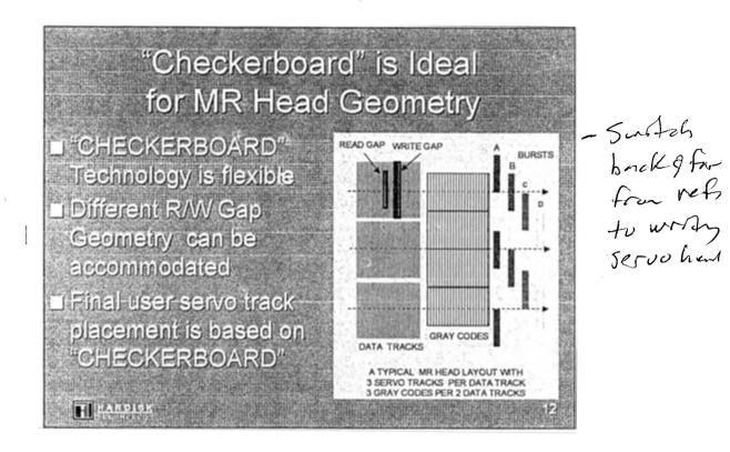
1) "CHECKERBOARD" Technology is well suited to MR heads due to the intrinsic temporary reference approach. For MR head technology it is very desirable to control squeeze such that track edges just touch.
