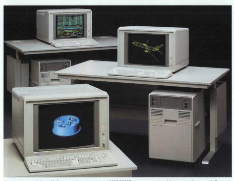
Each member of the 4120 Series is driven by an Intel 8286/80287 processor set and features a display with Dynamic Convergence; firmware with embedded commands for segment editing, segment subroutines and pick operations; a user interactive keyboard; and 4110 Series compatibility.
