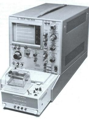
variable rate control is provided to set the test sequence at a rate which is best for the operator. New operators require more time per test, but with experience they will want to test at a faster rate. A front-panel switch or an optional foot switch advances the test in the manual mode.
