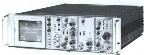
The R7903 requires only 5.25 inches of rack height in a standard 19 inch rack, It is fan-cooled and comes complete with slide-out chassis tracks.
