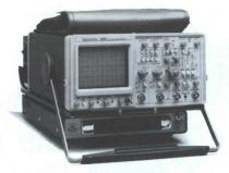
The Tektronix 2465 Oscilloscope with attached 1106 Battery Pack and 1107 Dc Inverter becomes a completely independent measurement package-readily transportable to remote sites where conventional ac power sources are not available.
