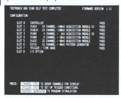
POWER ON: The configuration menu lists all modules in the DAS by slot location. A self-test verification is performed on each module with pass/fail indication. Bottom of screen indicates next step.
