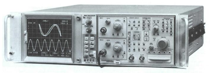
The 7D20 is used with 7000 Series oscilloscopes, such as the R7603, shown here, for rack installations. See pages 246 through 254 for details.
