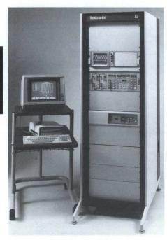
Tektronix MS 3201 Acquisition/Processing Measurement System using TEK SPS BASIC and a DEC PDP-11 Minicomputer.
