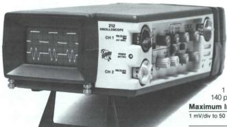
Display Modes - CH 1 only, CH2 only, or CH1 and CH 2 Chopped (chop rate ≈50 kHz) from 500 ms/div to 2 ms/div of time base, alternate from 1 ms/div to 5 µs/div of time base.
