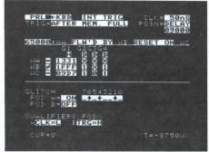
A 3-level trigger lets you define up to three events (A,B,C) which are then combined by using various operators to form the trigger sequence.
