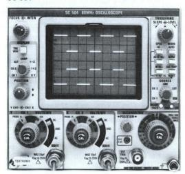
80 MHz Oscilloscope
