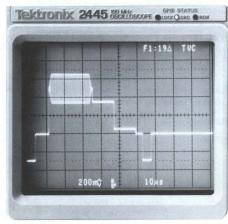
This sample waveform and CRT readout show a 2445's high-fidelity display of the Vertical Interval Reference Signal on Line 19, Field 1 with the television blanking-level clamp (TVC) engaged. The instrument used is also equipped with Option 10 (GPIB).
