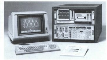
The MP 2201 Measurement Package (shown above) consists of 4105A, 4041, special software, plus MP 1201 Measurement Package (described on page 332). The MP 2101 Measurement Package (not shown) replaces the MP 1201 with the MP 1101 (described on page 332) and adds special software.
