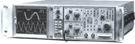
The R7603 requires only 5.25 inches of rack height in a standard 19 inch rack. It is fan cooled and comes complete with slide-out chassis tracks.
