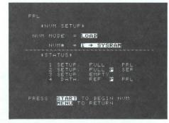
3 Setups and 1 memory (acquisition or reference) can be stored and protected in the nonvolatile memory.
