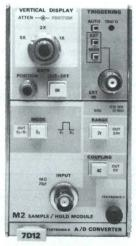
A/D Converter and Sample/Hold Module
