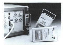
The printer interface consists of the combination of a ROM Pack and a COMM Pack. The 12RC01 Printer Support ROM Pack is used in combination with either the 1200C01 RS-232C COMM Pack (for printers with a serial interface) or the 1200C11 Parallel Printer COMM Pack (for printers with a parallel interface).
