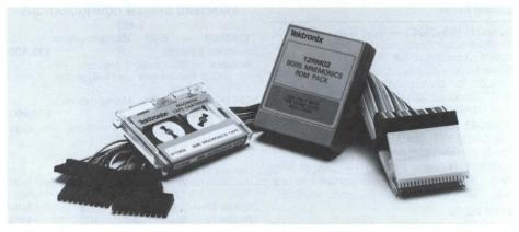
The Option 01 probe interface works with the mnemonics files on tape or ROM pack to support disassembly on the DAS 9100 and the 1240.
