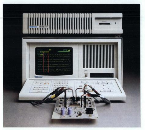
The color DAS 9129, the first logic analyzer with a color-coded CRT, is the undisputed leader in ease-of-use. Each menu is organized into color groups for faster interaction, better understanding, and fewer errors.
