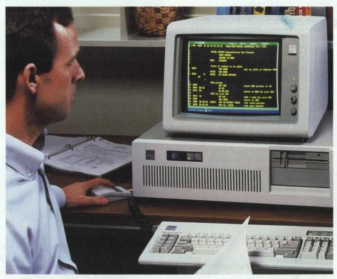
MicroLink™ FOR MICROCODE DEVELOPMENT — Tektronix's MicroLink provides an interface between the electronic design environment and the company's Microcomputer Development Systems. Using MicroLink, microcode can be developed on the TekStation™ and then tested using the Tek 8540 emulator and associated IC probe shown here.
