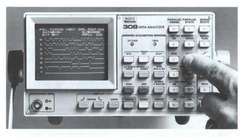
Serial — Synchronous or Asynchronous. Internal Clock for Asynchronous Mode Selectable Via Keyboard: 50, 75, 110, 134.5, 150, 200, 300, 600, 1200, 1800, 2400, 4800, and 9600 bits/second (baud rate). Internal Clock Accuracy: ±0.02%. External Clock for Asynchronous Mode: Up to 9600 baud. External Clock for Synchronous Mode: Up to 9600 baud.
