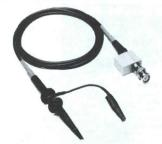
The P6125 is a low-capacitance, 5X attenuation passive probe specially designed for use with counter/timers. It makes possible more accurate time interval measurements of high speed logic signals. Five-times attenuation provides an optimum match between the counter input characteristics and the voltage levels of all common logic families. The low input capacitance permits acquisition of high frequency signals with minimum loading of the circuits under test.
