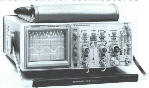
ference is improved over the standard 2235, and meets MIL-STD-461B part 4 requirements. It has adjustable graticule illumination as well as uncalibrated indicator lights for both the horizontal time base and the vertical channels. HF REJ and LF REJ filtering expand flexibility for trigger coupling.
