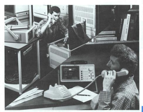
The 1240/1241 supports master/slave operation with the following configuration: A 12RC02 Master/Slave ROM Pack, a 1200C01 RS-232C COMM Pack and a modem.
