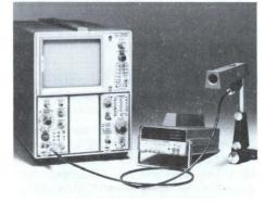
J16 probe used to measure pulsed light source.
