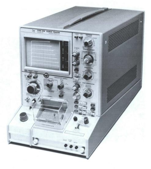
The Tektronix 576 Curve Tracer System continues to hold the title "standard of the industry". The 576 accepts three different test fixtures: the Standard Test Fixture, 172 Programmable Test Fixture (see page 396), and the 176 Pulsed High-Current Fixture (see page 397). The 576 is an excellent general purpose curve tracer system that performs well in applications where high-current testing is required.
