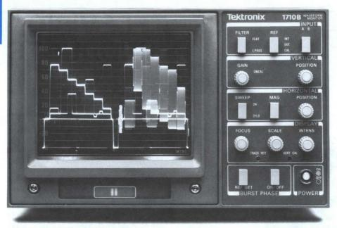
1710B Waveform Monitor-Dual Filter Display
