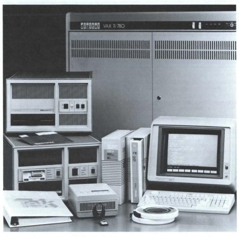
can be easily upgraded within the same mainframe to an LSI-11/73 CPU, 55 Mbyte of hard disk, 512 kbyte or 1 Mbyte of RAM memory, a GPIB interface for disk backup, and four or eight user ports. Each 8561 user port can support either a standard CRT terminal, a Tektronix 410X Color Terminal, or a Tektronix 8540A or TekMate Microprocessor Support Systems designed specifically to handle hardware/software integration tasks through real time emulation.
