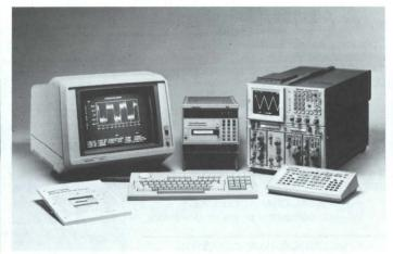
The MP 2401 Measurement Package consists of a display monitor, 7D20T, 4041, 4105A, and software.
