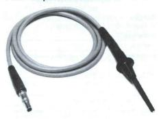
The P6601 Probe is a temperature measuring device designed to operate with the DM 502A and DM 501A Digital Multimeters. The temperature sensing element consists of a thin-film platinum resistor on the tip of the probe. Measurements are made by touching the probe tip to the surface whose temperature is in question. The thermal signal is transmitted to the associated digital multimeter through a two-conductor cable.
