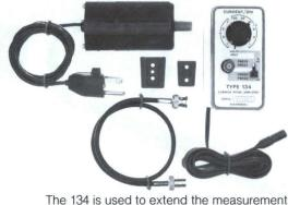
capabilities and sensitivity of the P6021 or P6022 Current Probes. A Current/Div switch provides calibrated current steps from 1 mA/div to 1 A/div (with the oscilloscope or plug-in unit adjusted for a deflection factor of 50 mV/div). A passive termination is not required when using a 134 with a P6021 or P6022.
