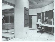
E-Beam pattern data being reviewed prior to generation of a photomask. Class 10 MEBES III write room is at left.
