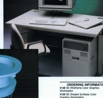
An 80286/80287 processor set drives each unit and provides rapid data communications—at rates up to 38.4 kbaud. Both units come with 288 kbytes of RAM, expandable to 800 k. The 4128 offers 4-bit planes and the 4129 is equipped with 8-bit planes as standard. Both share a new, high-resolution 1280 x 1024 in-line display with dynamic convergence.
