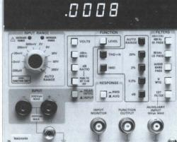
AA 5001 PROGRAMMABLE DISTORTION ANALYZER
