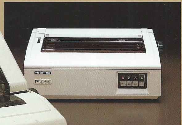
Printer choices include Toshiba's advanced P1350 (132 column) and P1340 (80 column) Three-In-One dot matrix printers.
