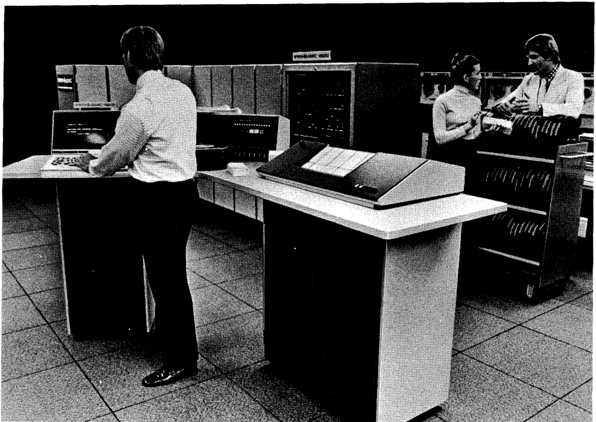
Figure 1-1. The Central Processor and Operator's Console
