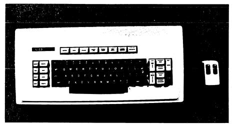
Photo 2: The Star keyboard and mouse. Note the two buttons on top of the mouse.
