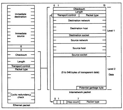
2. An internet packet (16 bits wide) is encapsulated in an Ethernet packet.
