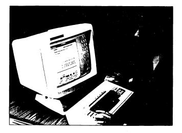
Figure 1—A Star workstation showing the processor, display, keyboard and mouse
