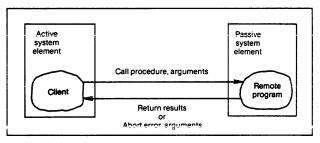
7. The Courier remote procedure call protocol covers the manner in which a client invokes operations from a remote program. It simply calls for a procedure and expects the results to be returned or the operation to be aborted.
