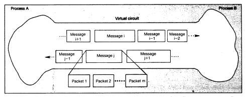
3. A connection is a transient association between two processes that allows messages to flow back and forth. The sequenced packet protocol allows packets to be assembled into messages and removes the limitation on packet size at lower architectural levels.
