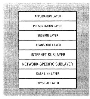
Figure 2. Enhanced ISO open systems interconnection reference model with seven layers.
