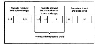
5. A flow-control window is set up by the sequenced packet protocol, using its sequence, acknowledgment, and allocation numbers. The wider the window, the fewer the number of interactions between source and destination during message transmission.
