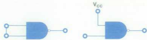
Fig. 2. Configurations of a NAND gate used as an inverter.
