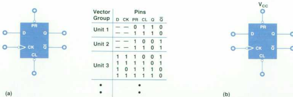
Fig. 5. (a) D-type flip-flop and library test sequence. (b) Use of flip-flop on board under test. For this topology, the library test is modified by removing test vector unit one.
