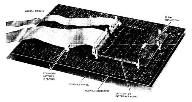
Figure 3-7. Tester Assembly
