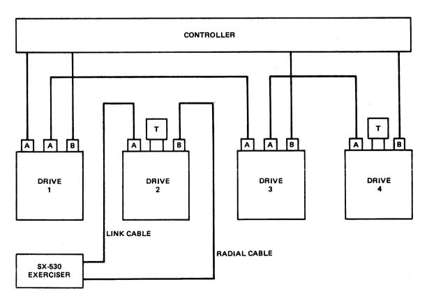
Figure 3-2. Typical Subsystem with Drive 2 Removed for Testing
