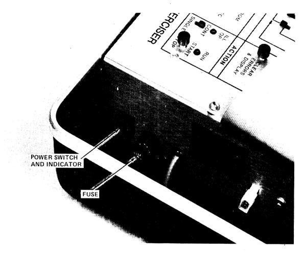
Figure 3-6. Power Switch and Indicator Location
