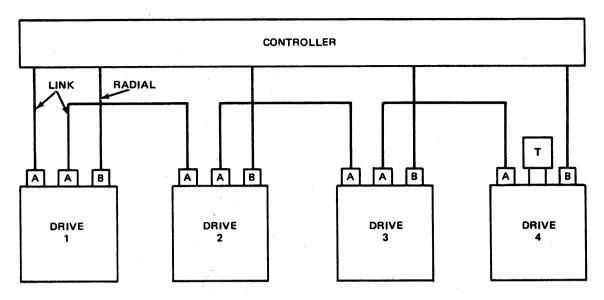
A = LINK OR DAISY CHAIN CABLE CONNECTION B = RADIAL CABLE CONNECTION
