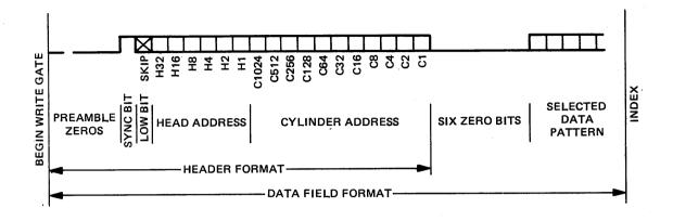
Figure 3-4. Header and Data Field Detail
