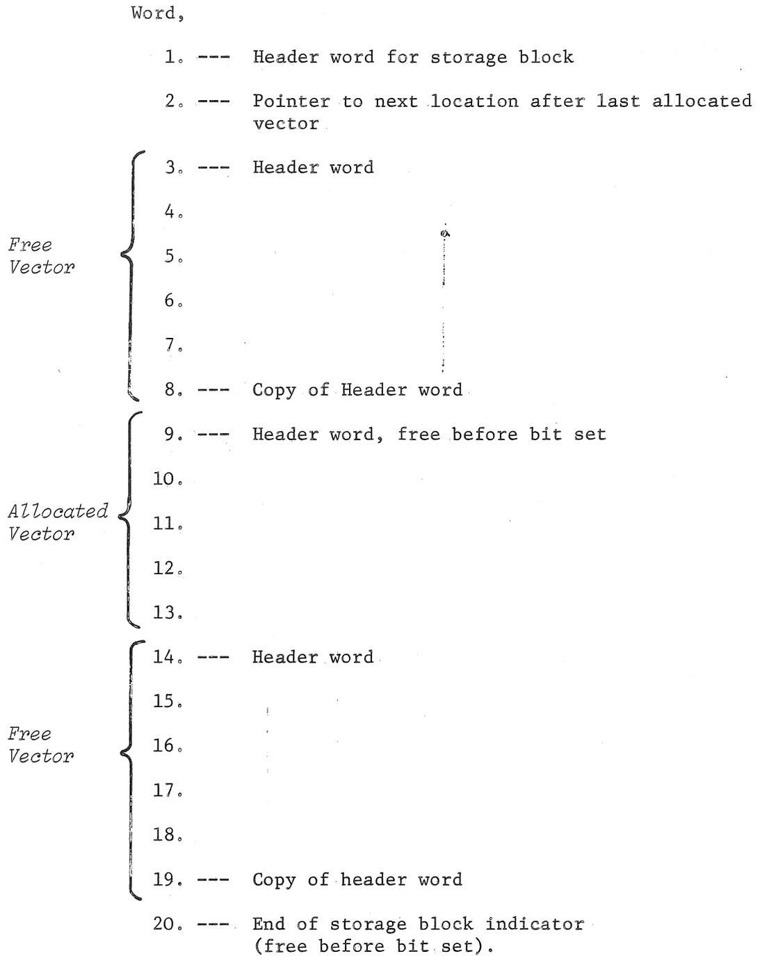
Figure 1. Typical Contents of a Storage Block
