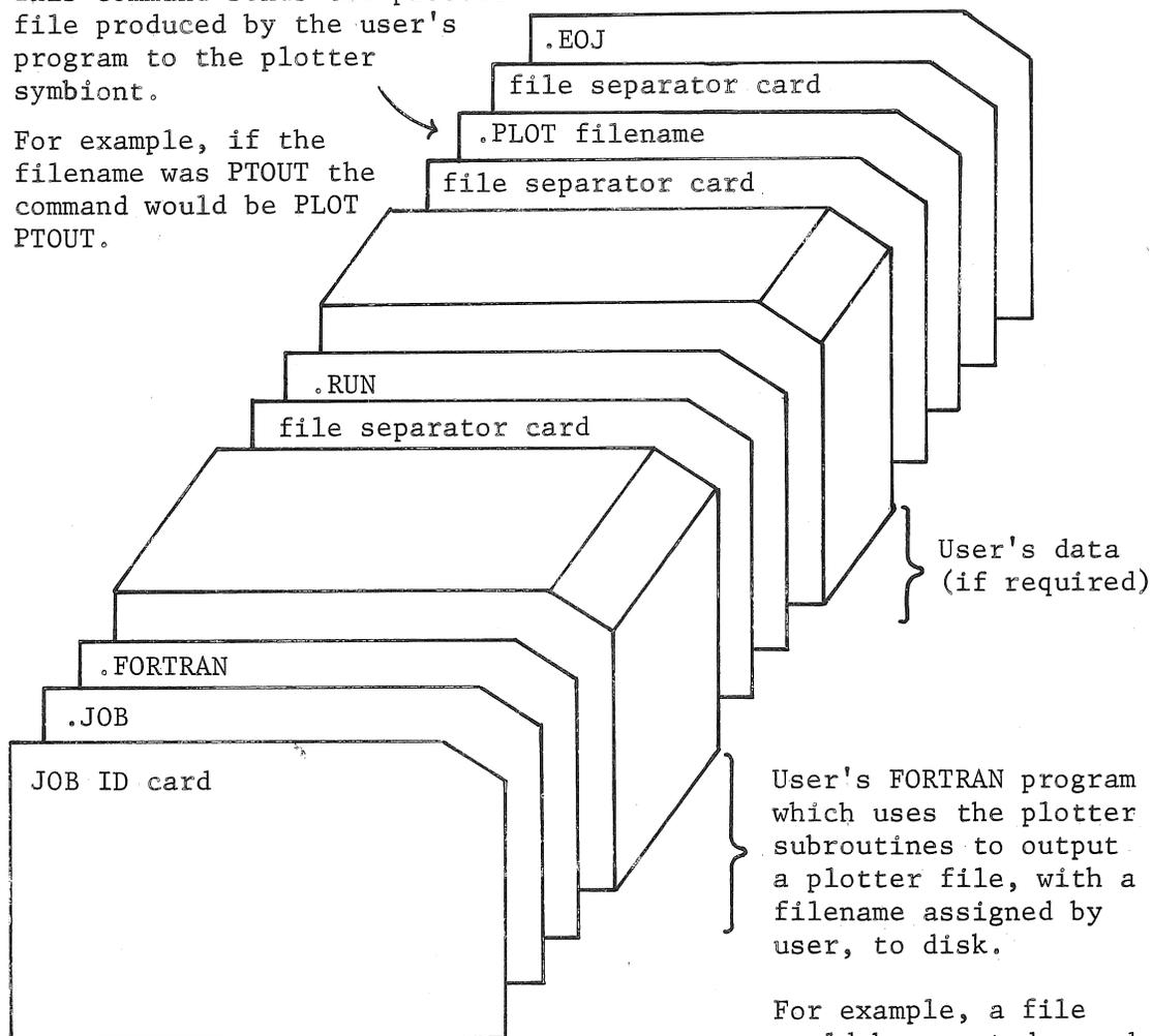
User's FORTRAN program which uses the plotter subroutines to output a plotter file, with a filename assigned by user, to disk.
