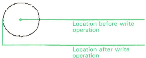
The same is true for arcs. Depending on the form of the curve command, GIGI leaves the current location either at the center of the arc or on the arc perimeter, as shown in Figure 7-6.
