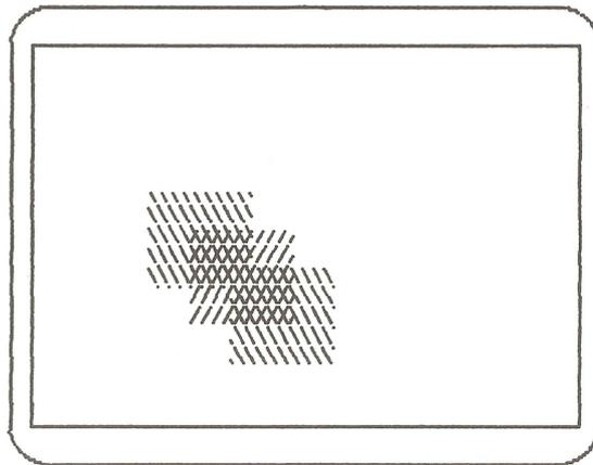
In this mode, GIGI changes a pixel bit to 1 if the writing pattern bit is 1 and does not change the pixel bit if the writing pattern bit is 0. Thus if a pixel bit is 1, it stays 1; if a bit is 0, it is changed to 1 only if the writing pattern bit is 1.
