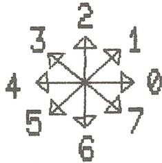
You can draw lines (with the V command) or move the current location (with the P command) using one of these directions rather than a screen location.
