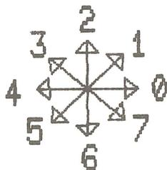
Screen movement is relative to the current cursor position. GIGI accumulates partial offsets and moves the screen when a sufficient number of values is entered.
