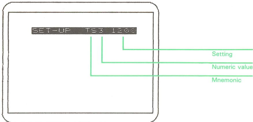
In the sample screen in Figure 2-1, the first two characters are the mnemonic for the set-up parameter, in this case TS is the mnemonic for Transmit Speed. The mnemonic is followed by a numeric value which specifies the setting for the keyword; in the example, TS3 sets a transmission speed of 1200 baud. The value following the numeric keyword setting, 1200 in the example, shows the meaning of the numeric setting.
