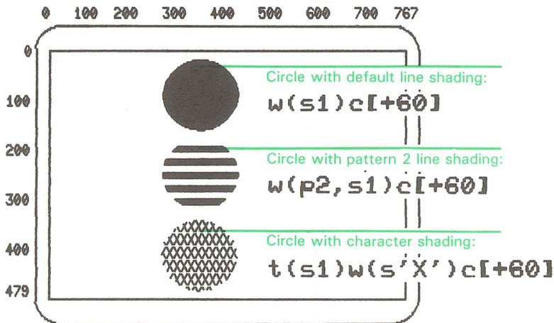
Such shading can be used for area fill, but GIGI cannot automatically ensure that arbitrary areas are completely and correctly filled; you must ensure that the correct reference line or lines are specified to achieve the desired fill effect.
