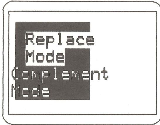
In complement writing, if the pattern bit is 0, GIGI does not change the pixel bit being written. But if the pattern bit is 1, GIGI changes the bit being written to 1 if it is 0, or to 0 if it is 1.
