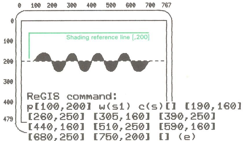
As you can see in Figure 8-1, the shading reference line is set to the current location [,200]. GIGI executes the curve command shown in the figure and shades the area between the reference line and the line being drawn. In Figure 8-2, below, the same curve command is executed but the shading reference is set to [,300] by the explicit reference.
