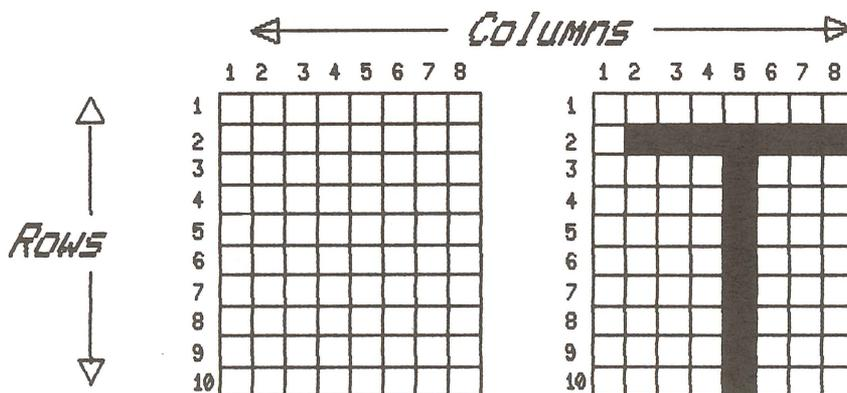
The image that comprises the letter T is created by setting pixels in the cell. When the letter is displayed, dots (i.e. the pixels that are set) are drawn and make the image in the cell look like the letter T. The image that you create when you set pixels in the character cell is called a text pattern.
