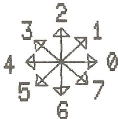
The length of the line drawn is a single point unless you set the *direction* length. Set *direction* length permanently using the Writing command multiplier (M) option; set the length temporarily using the temporary writing controls described below.
