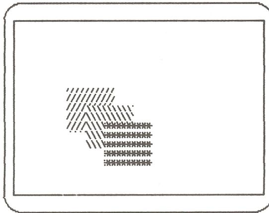
Replace writing forces the pixel bit to be the same as the pattern bit (either 0 or 1) regardless of the current value of the pixel bit.
