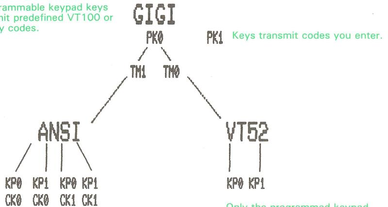
Both the programmed keypad and the cursor keys can be programmed using VT100 key codes.
