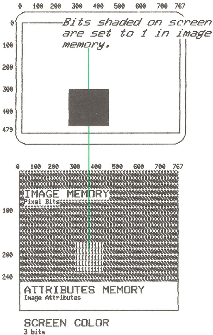
In Figure 11-1, the image drawn on the screen maps to an image in video memory. You can see that bits set to 1 in image memory form a rectangle; GIGI uses the attributes in image attribute memory to display pixels corresponding to these bits. For example, the color attribute for images might be yellow. The other bits are 0's; GIGI uses the attributes set for screen attribute memory to display pixels corresponding to these bits.
