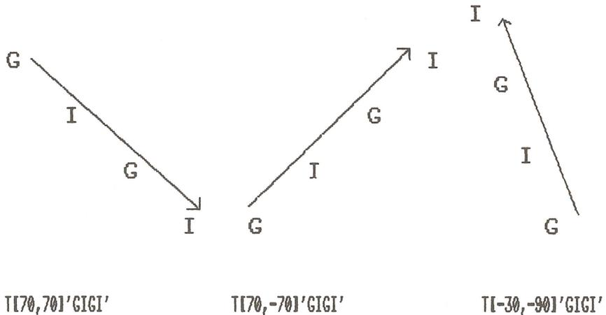
The first example, ReGIS command T[70,70], spaces each new character 70 pixels across and 70 pixels down. The second example, ReGIS command T[70,-70], begins each new character 70 pixels across and writes up, using -70 as the vertical character spacing. The third example, T[-30,-90], shows GIGI writing backwards and upward.
