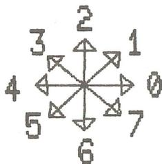
Offset directions are used with the P, V, C, and T ReGIS commands to move the graphics cursor before display of graphics objects, for example a text string.
