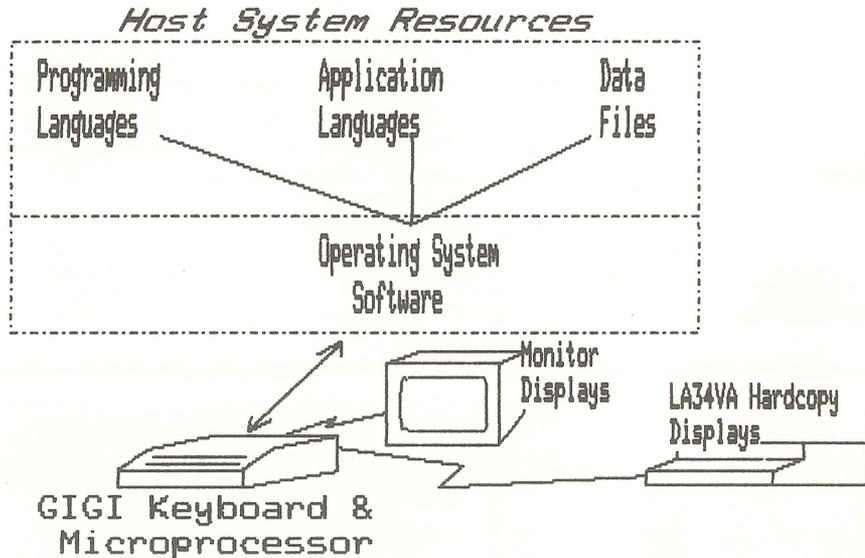
The document *GIGI Terminal Installation and Owner's Manual*, Order Number EK-VK100-IN, describes GIGI's terminal hardware components in detail and tells you how to operate the terminal; the document *DECwriter IV Graphics Printer User Guide*, Order Number EK-L34RO-UG, describes the LA34VA graphics printer and how to operate it.
