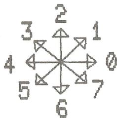
*Direction* is relative to the current character direction. Depending on the settings for character height, width, and direction, spacing for characters is in 1/2-width row increments and 1/2-height column increments. This provides a convenient form for superscript/subscript.
