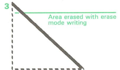
The first line of ReGIS code above sets the shading reference to [,400] and enables shading, W(R,S1). The second line of code draws a single line from [400,200] to the location 200 down and 200 to the right. However, because shading is enabled, GIGI appears to be drawing a triangular shape. Line 3 of the code enables erase mode writing and line 4 draws another single line but, while drawing in erase mode, GIGI erases the part of the triangle which was previously shaded.
