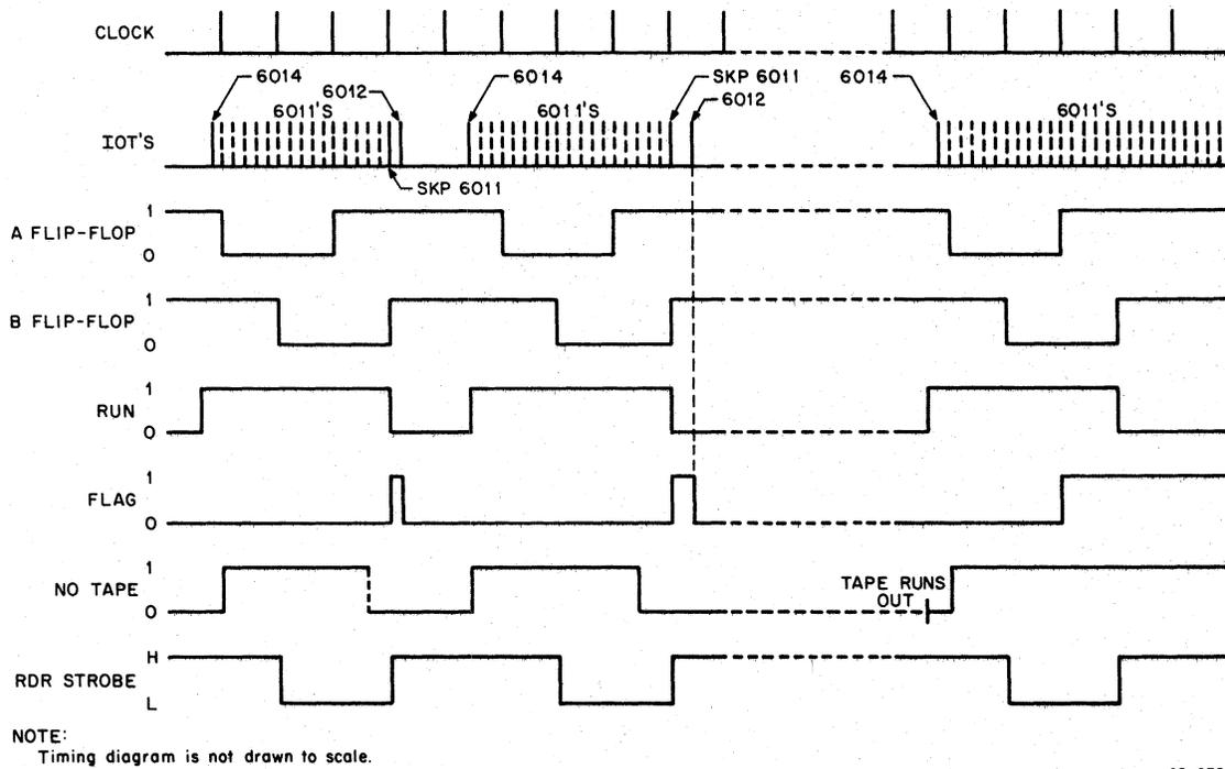
Figure 4-4 Tape Reader Timing Sequence for PA68F
