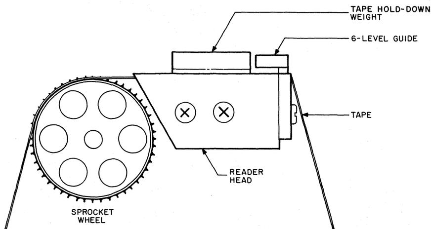
Figure 5-6 6-Level Guide and Reader Head Adjustment
