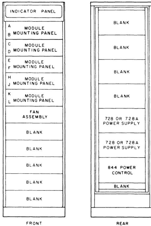
Figure 1-1 DF10 Data Channel, Assembly Locations
