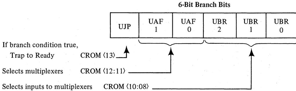
The three UBR bits are applied to each of the six multiplexers and uniquely specify one of the inputs to the multiplexer. If UBR bits 2, 1, and 0 are all 1s, the multiplexer output goes to 0, which indicates no modification takes place. For all other combinations, the multiplexer output goes to a 1 if the selected branch condition is true. The UAF bits specify the multiplexer(s) as follows:
