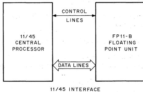
Figure 2-1 11/45 Simplified Interface Diagram
