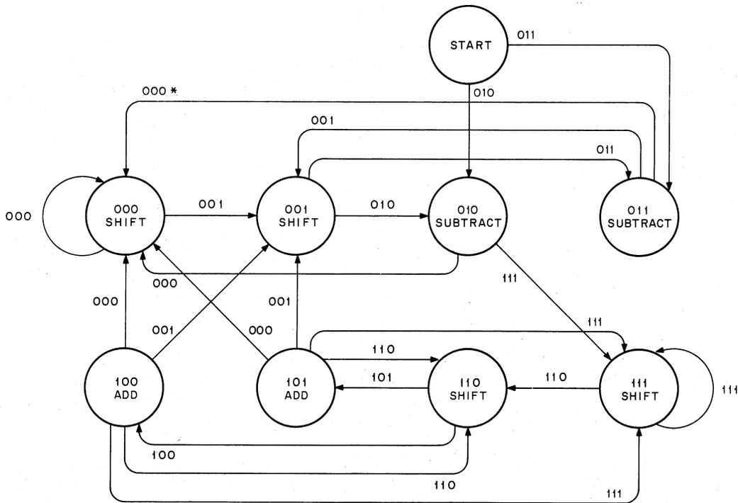
\* Three digits shown throughout state diagram refer to bits AR59, 58, and 57. For example,
