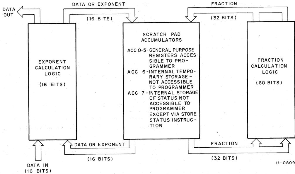
Figure 1-2 FP11 Simplified Block Diagram
