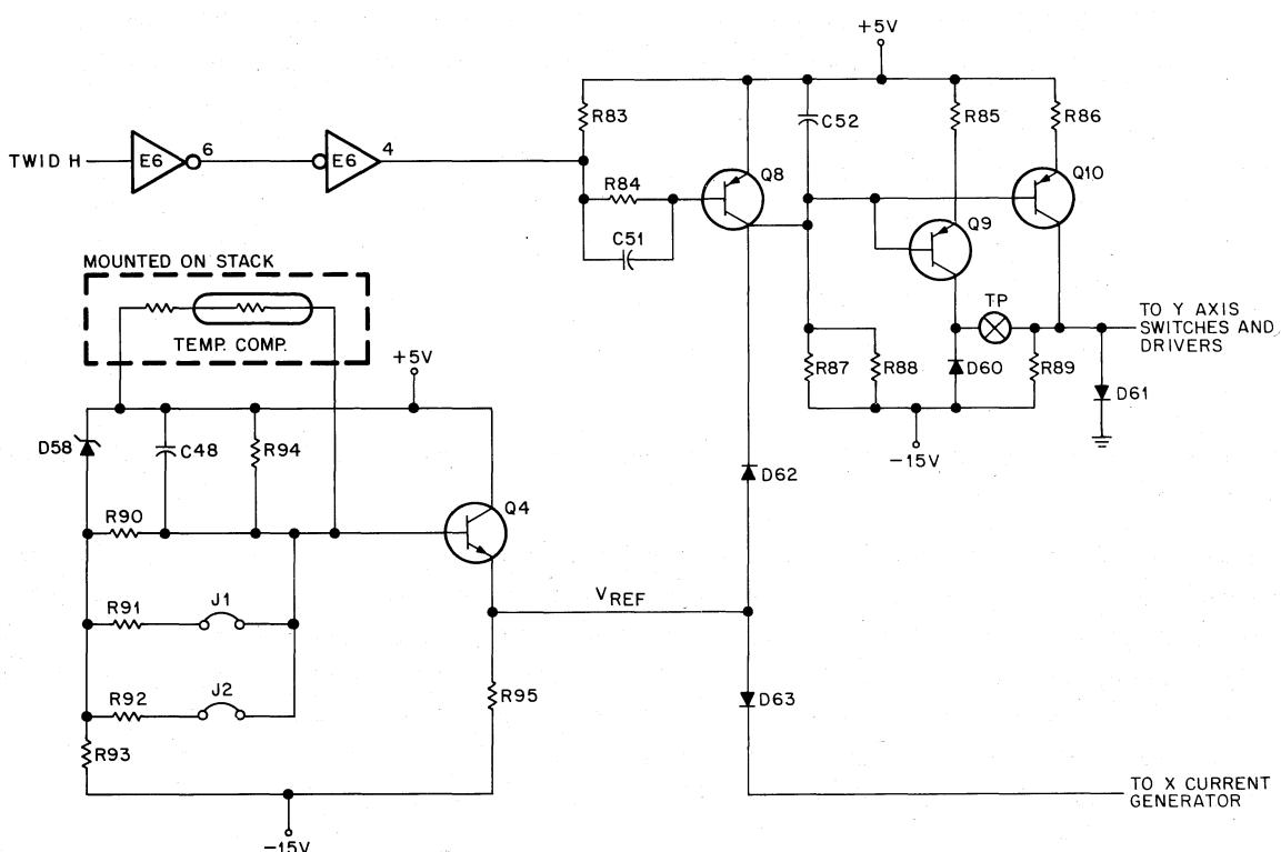
Figure 2-16 Y Current Generator and Reference Voltage Supply
