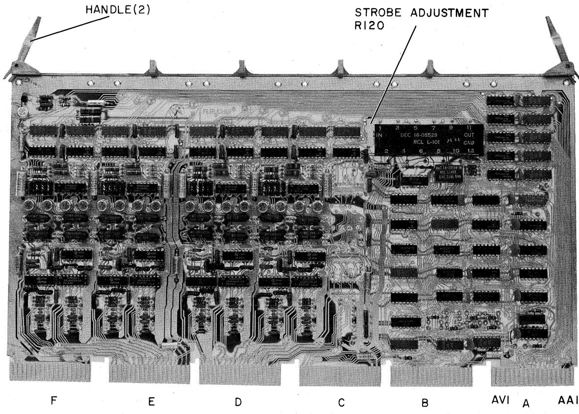
Figure 1-1 Component Side of Control Module G110
