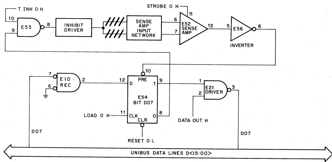
Figure 2-14 Interconnection of Unibus, Data Register,
