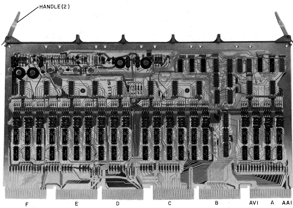
Figure 1-2 Component Side of Driver Module G231
