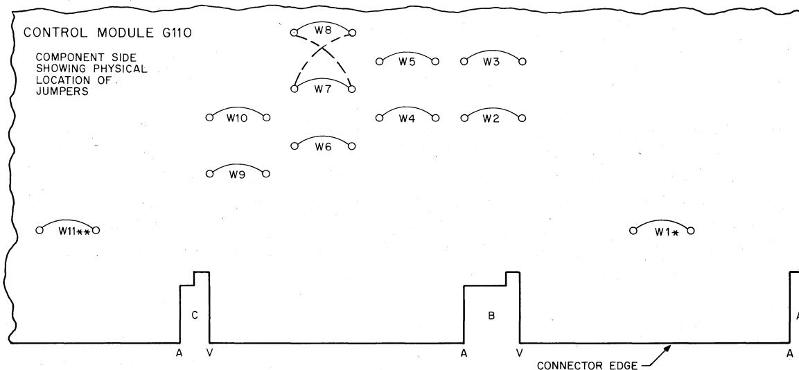
\*Jumper W1 is for test purposes only. It must be installed for normal operation.
