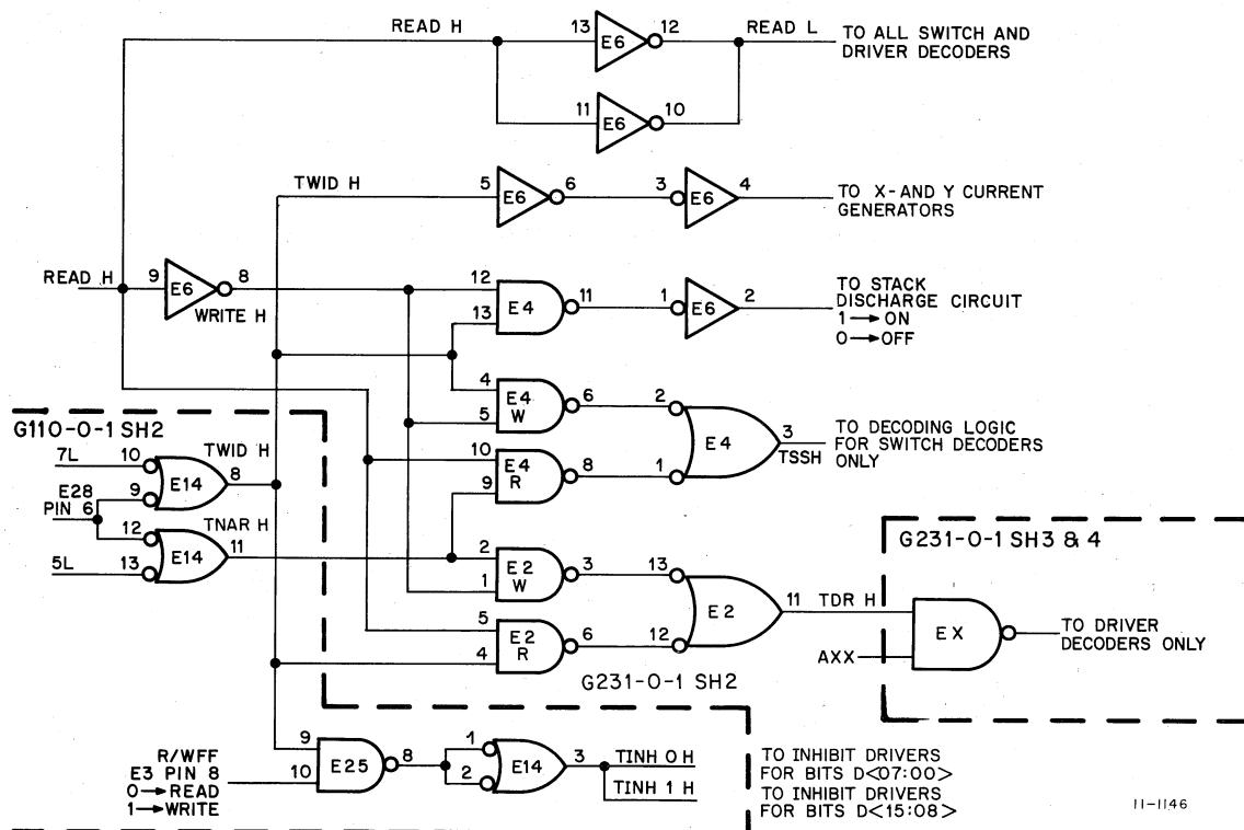
Figure 2-22 TWID H and TNAR H Control Logic
