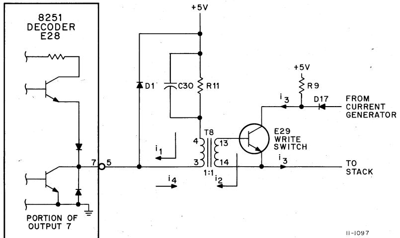
Figure 2-11 Switch or Driver Base Drive Circuit
