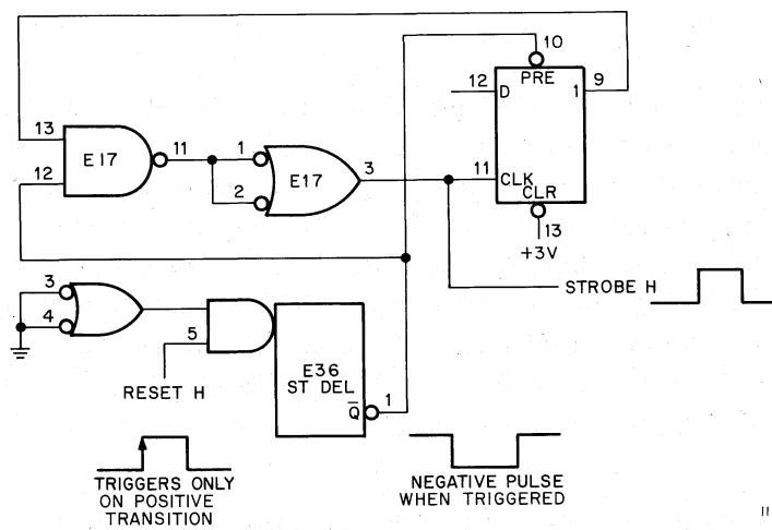
Figure 2-26 Strobe Generating Circuit and
