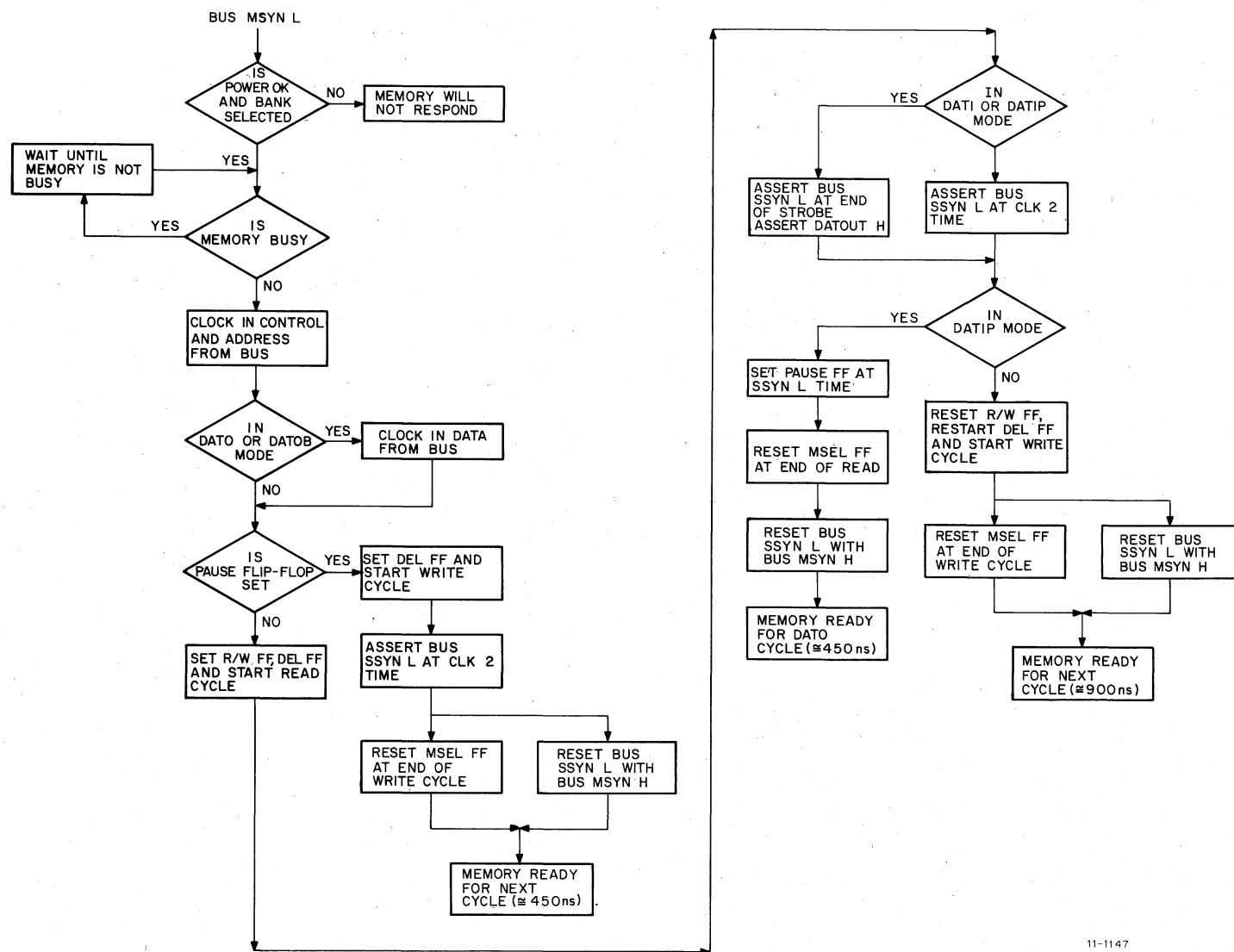
Figure 2-27 Flow Chart For Memory Operation
