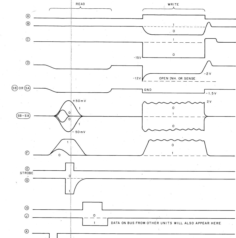
Figure 3-3 MM11-L Sense/Inhibit Waveforms
