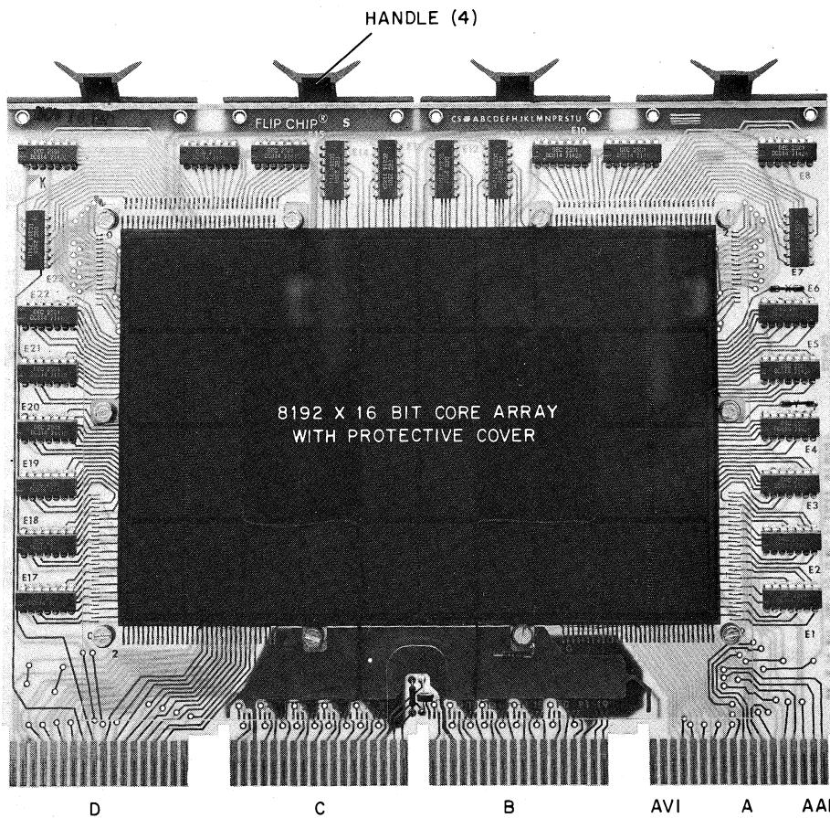
Figure 1-3 Component Side of Stack Module H214
