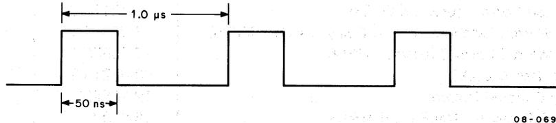
Figure 5-2 Scanner Clock Waveform
