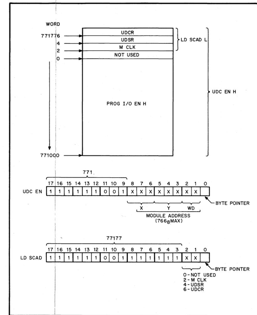
Figure 3-2 Address Selector Logic
