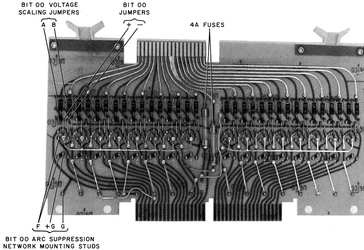
Figure 4-53 Location of Jumpers and Component Mounting Studs (W402)
