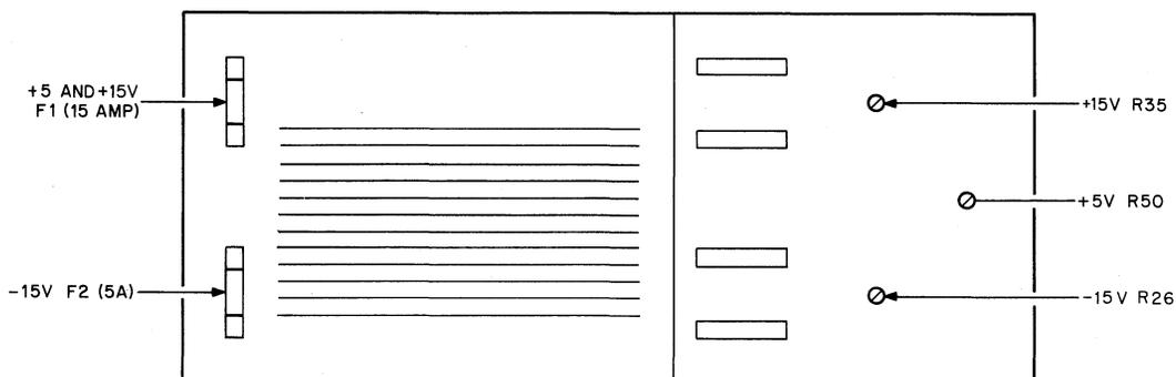
Figure 5-1 H740 Power Supply Fuses and Adjustment Controls
