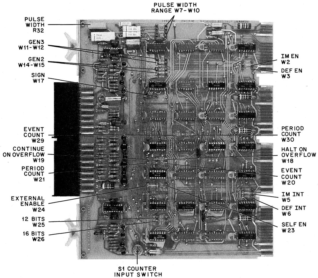
Figure 4-28 Location of Jumpers and Input Switch (W734)
