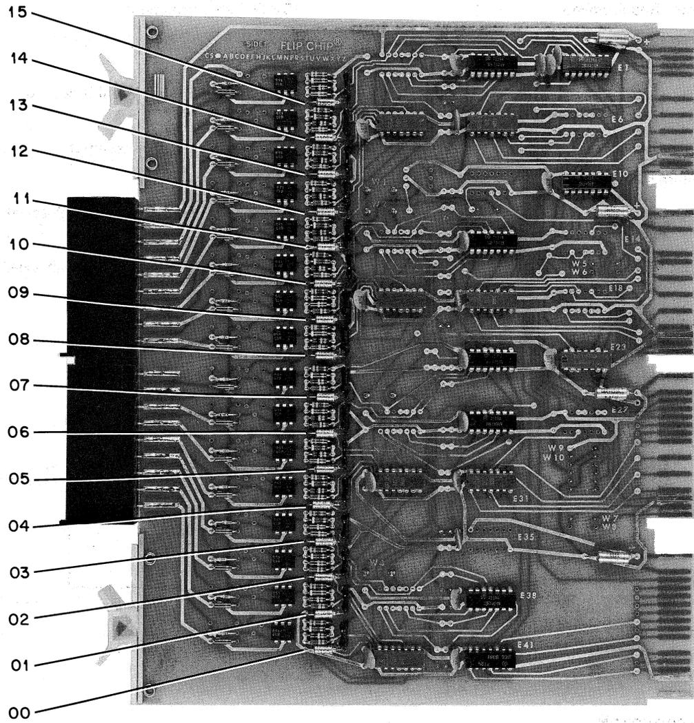
**Figure 4-13 Location of Bit Response Time Capacitors (W741)**
