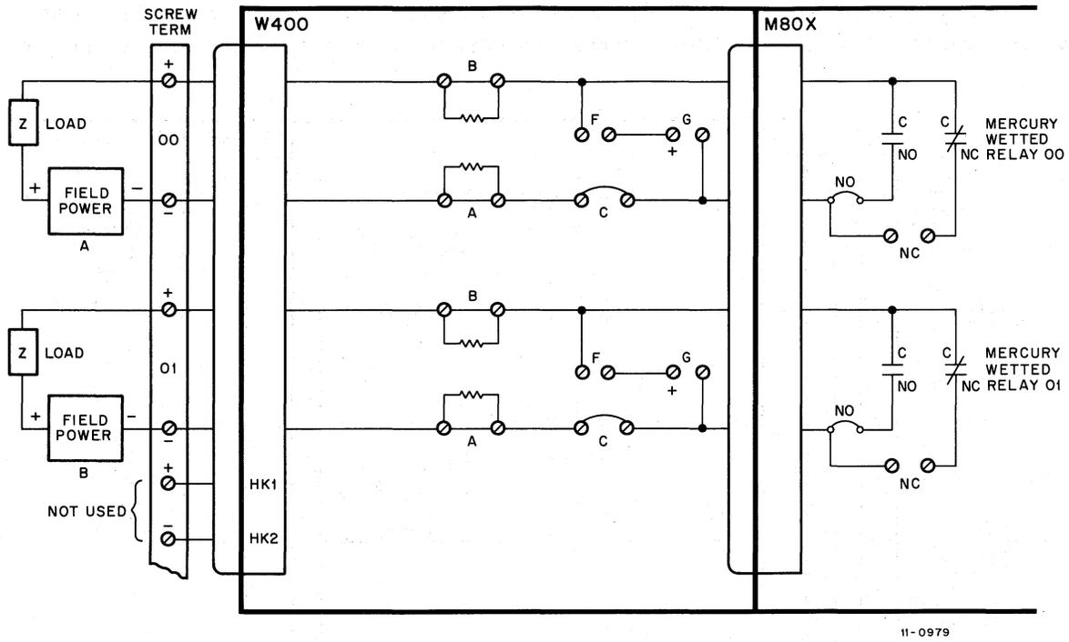
Figure 4-31 Isolated Power for Load Switching, Wiring Diagram
