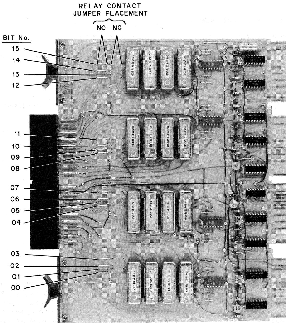
Figure 4-22 Location of Bit Relay Contact Jumpers (M805)
