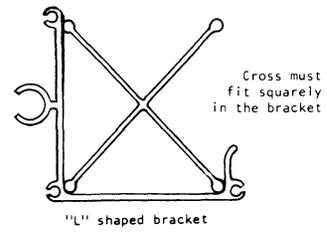
Figure 3-2 Inserting Cross in Roll Paper
