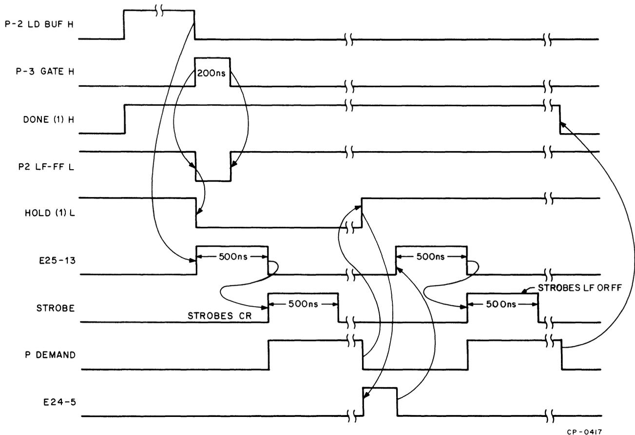
Figure 4-7 FF and LF Timing Diagrams
