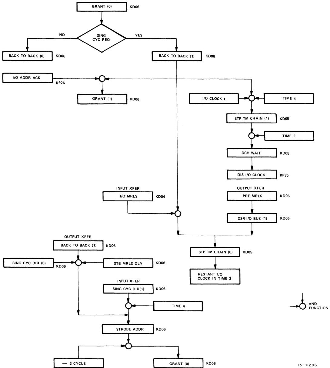
Figure 4-11 Single Cycle Back-To-Back Transfer, Detailed Flow Chart
