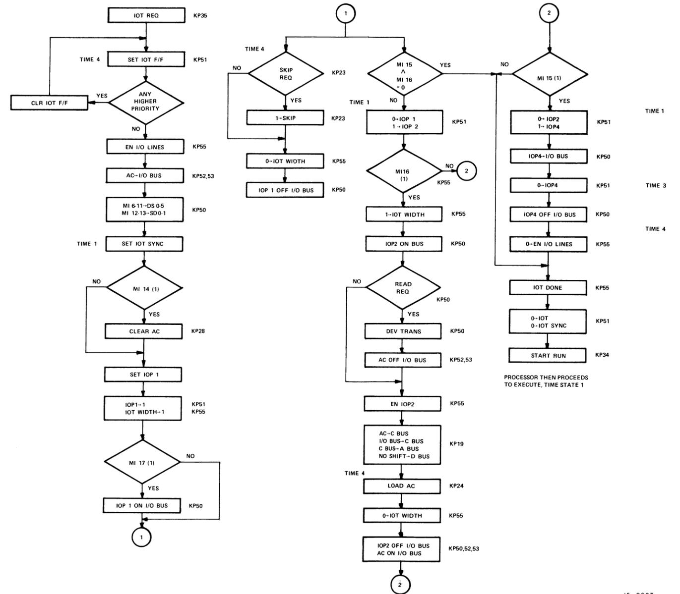
Figure 4-4 IOT Flow Diagram
