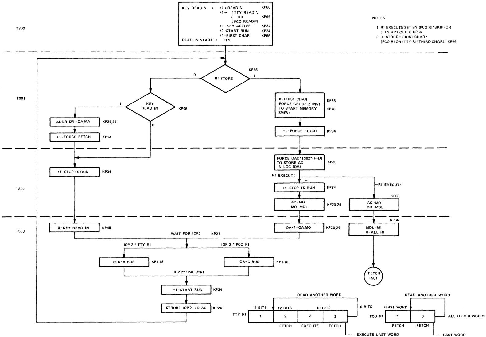
Figure 3-4 Read-In Flow Diagram
