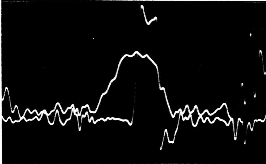
Figure 7-8 MEM Strobe/Sense Amp Output
