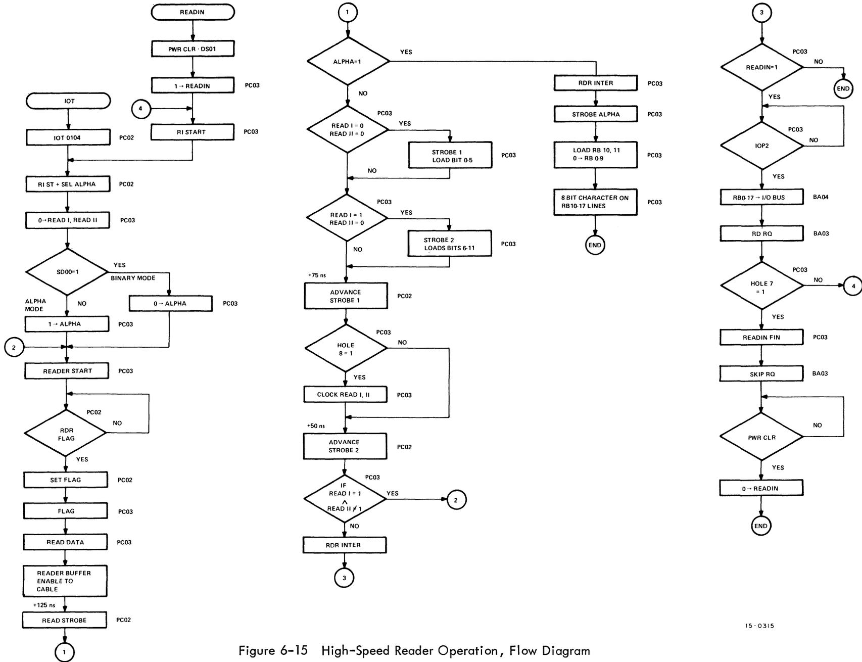
Figure 6-15 High-Speed Reader Operation, Flow Diagram
