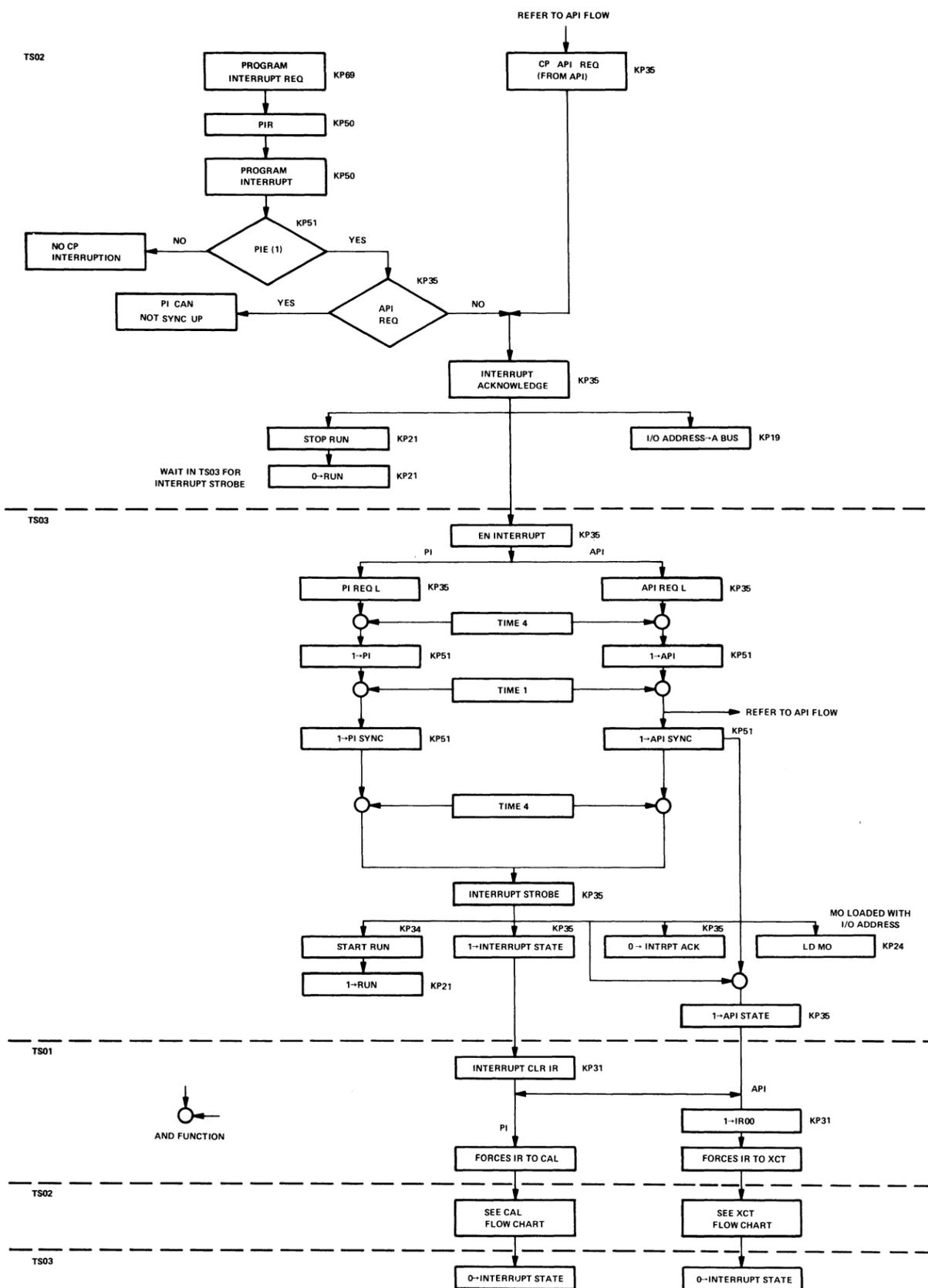
Figure 6-10 API/PI/Central Processor Flow Diagram
