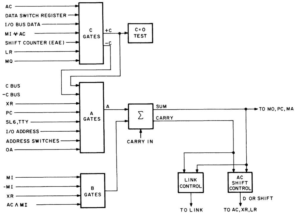
Figure 3-1 CPU Bus Structure
