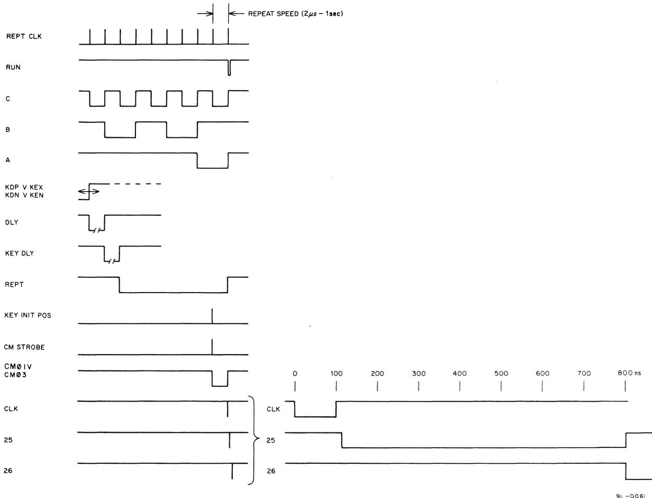
Figure 7-1 Initial Set-Up DEPOSIT or EXAMINE Timing
