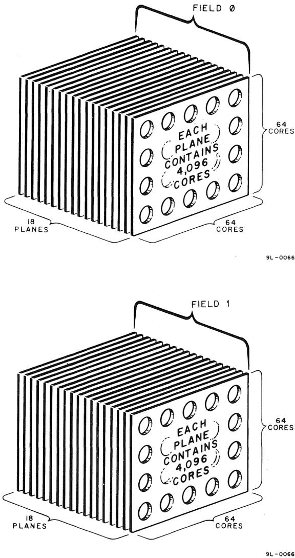
Figure 6-2 Core Memory Stacking Arrangement (Theoretical)
