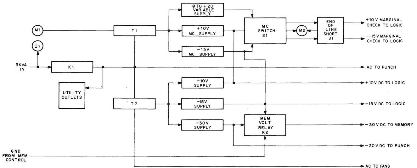
Figure 7-4 Power Supply 712, Block Diagram
