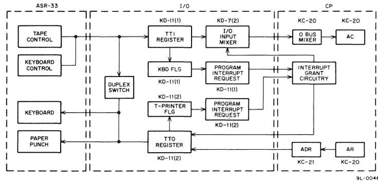
Figure 9-2 Basic I/O Data Transfer, Functional Diagram
