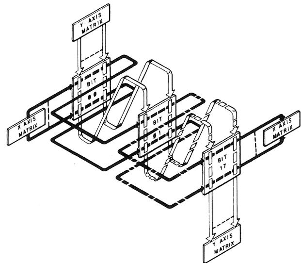
Figure 6-5 X and Y-Axis Selection Scheme for 18 Planes
