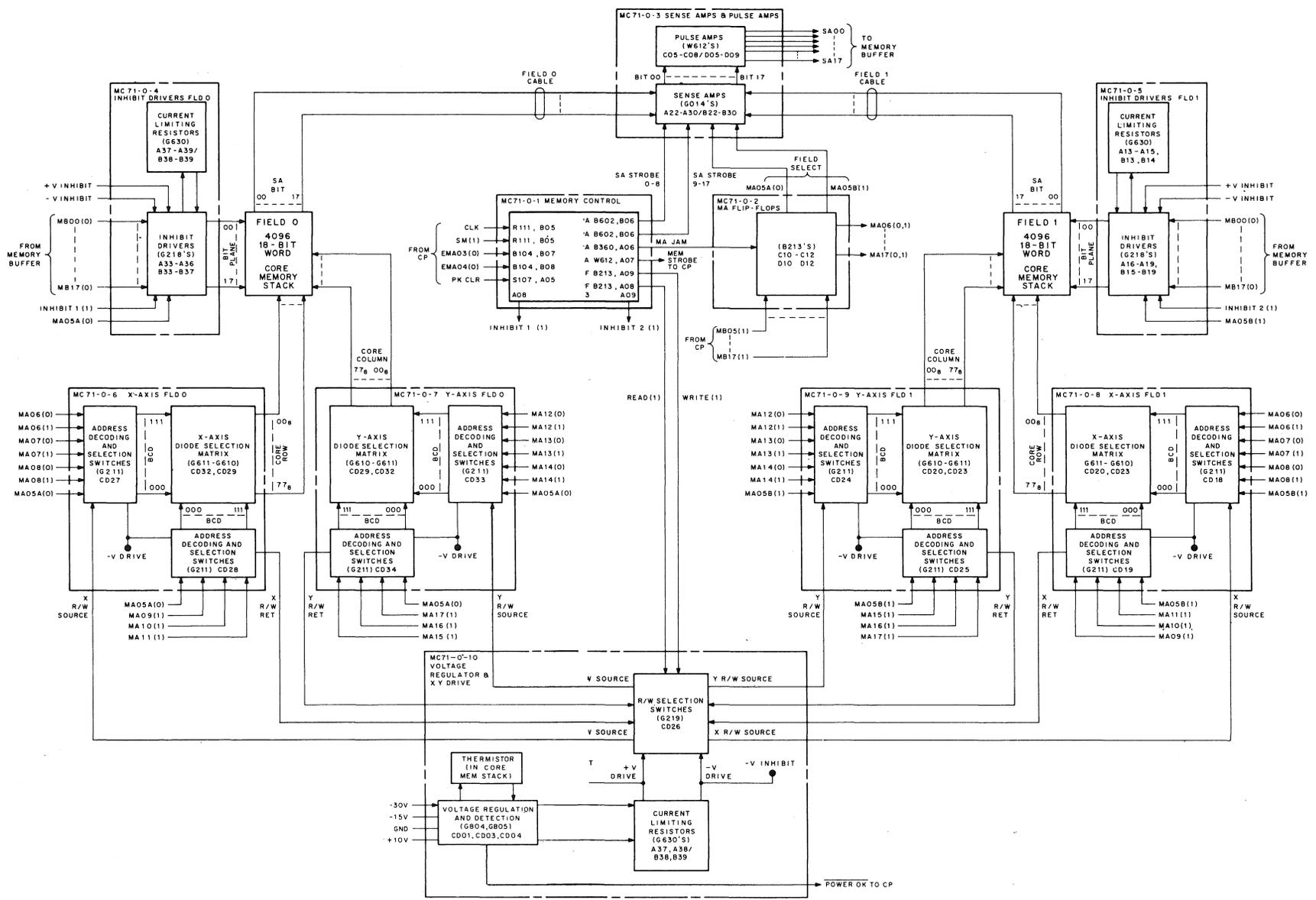
Figure 6-3 MC71A Core Memory System Block Diagram
