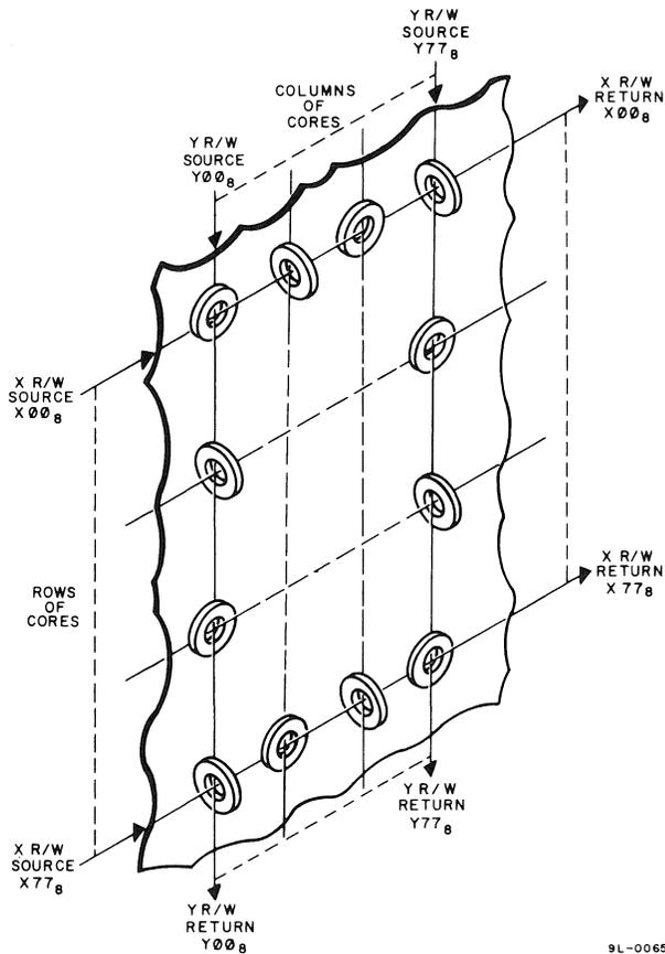
Figure 6-4 Core Row and Core Column Selection
