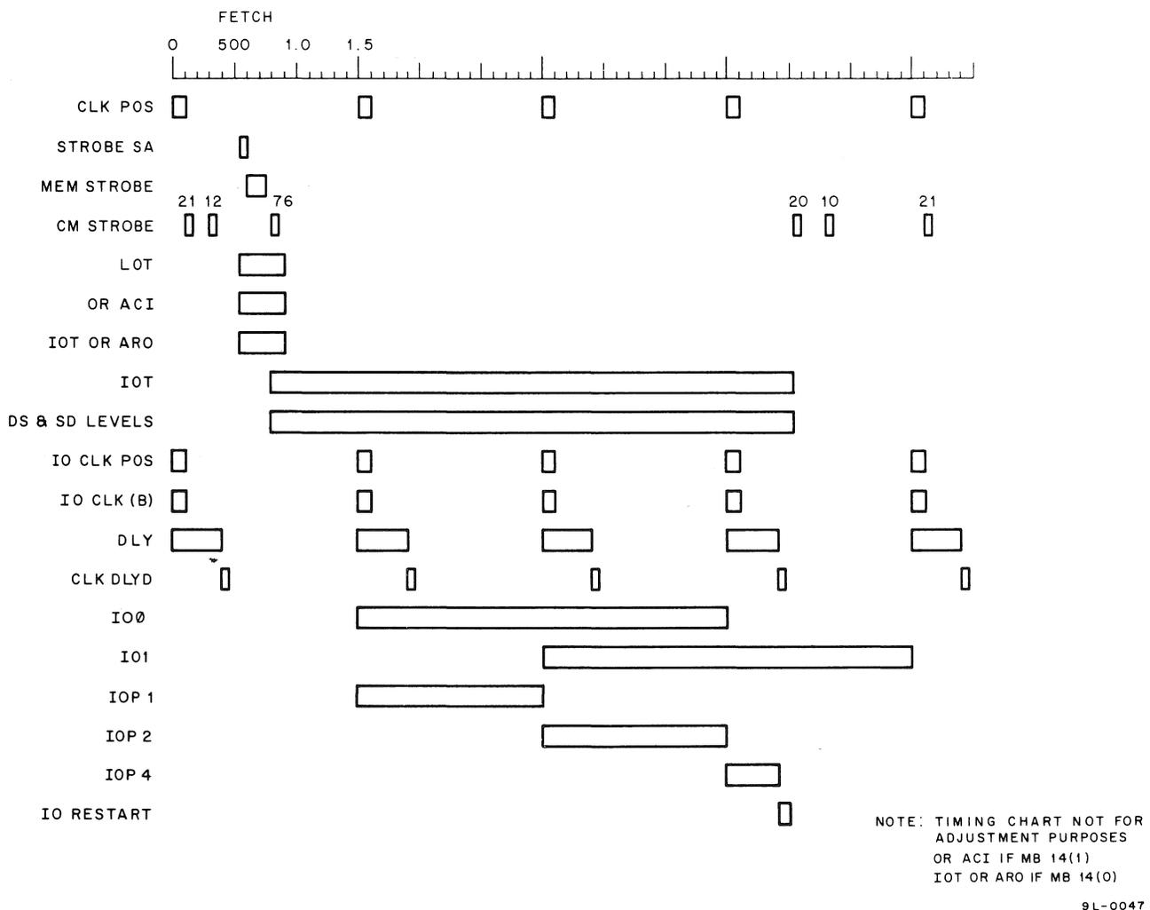
Figure 5-11 IOT Timing
