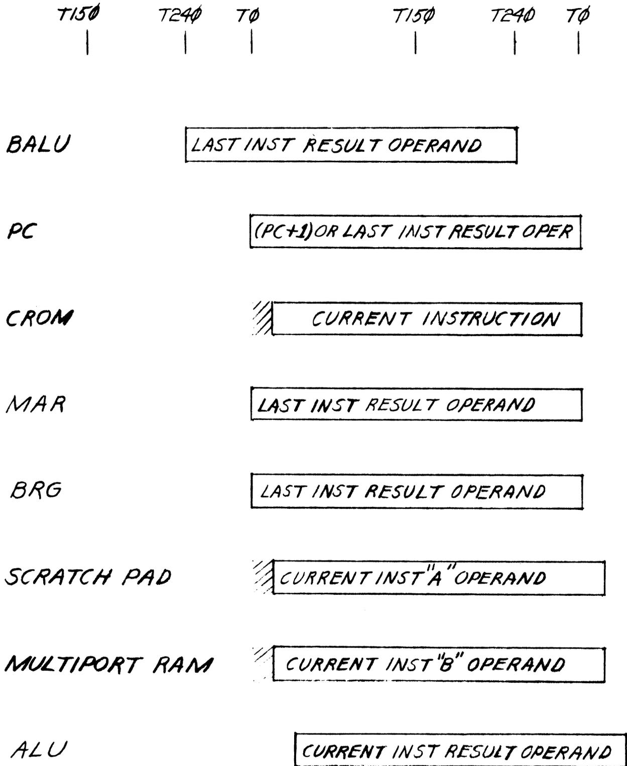
Figure 4-2 Microprocessor Register Timing
