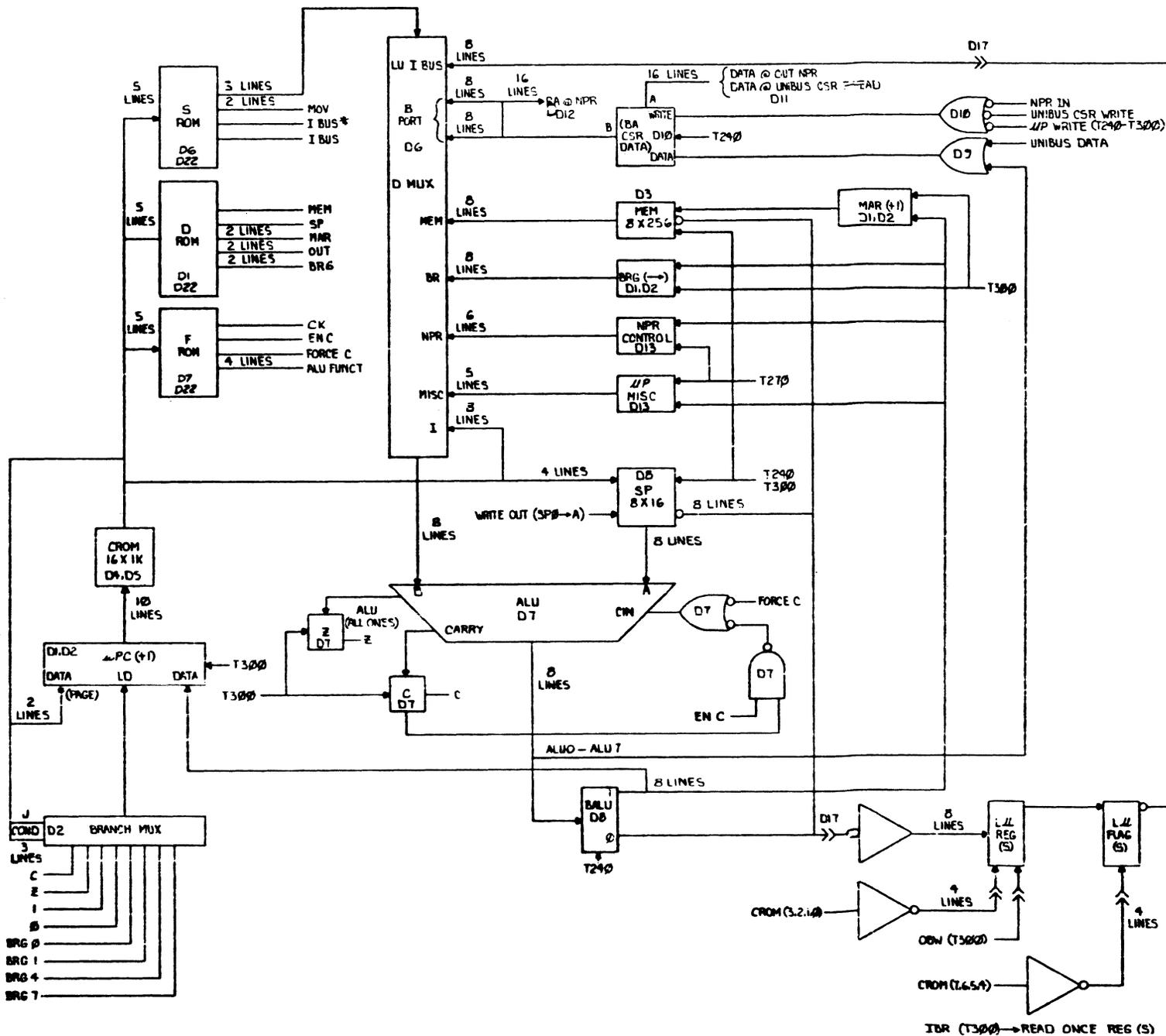
Figure 4-1 Microprocessor Block Diagram
