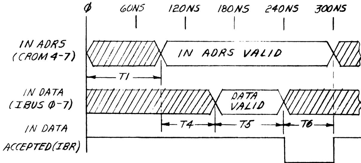
Figure 4-21 Typical Input Bus Timing
