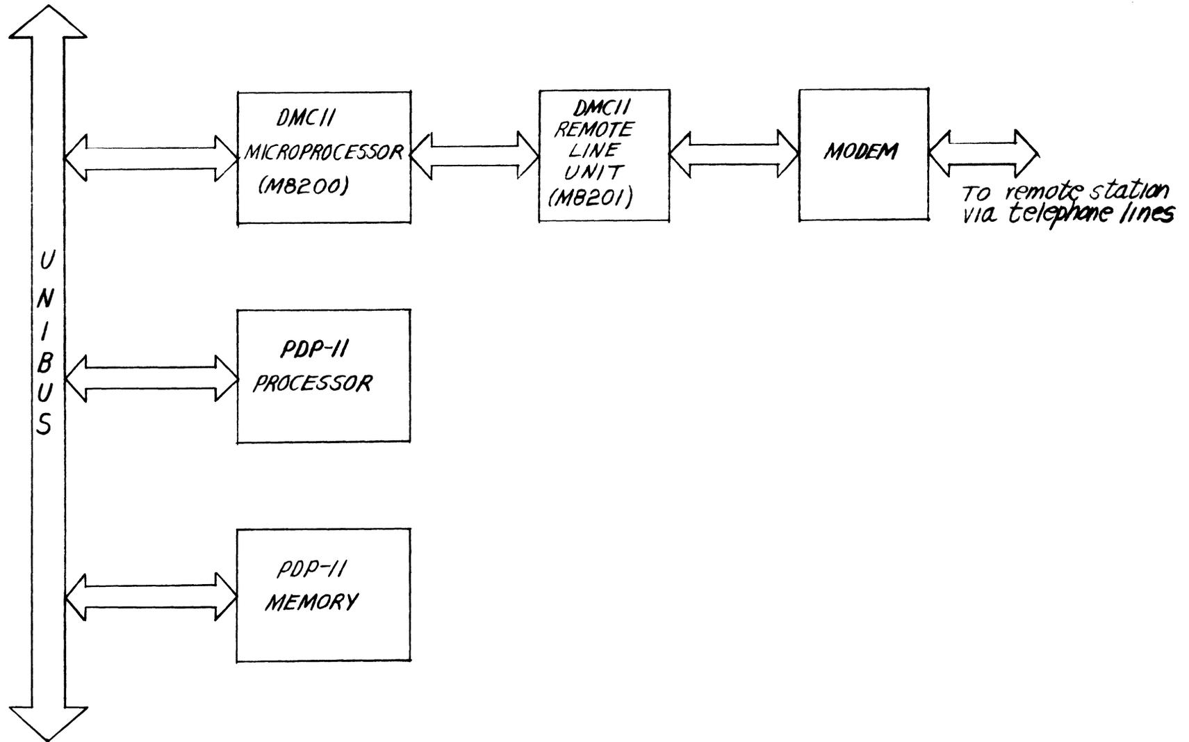
Figure 1-1 DMC11 Remote Line Unit Interface
