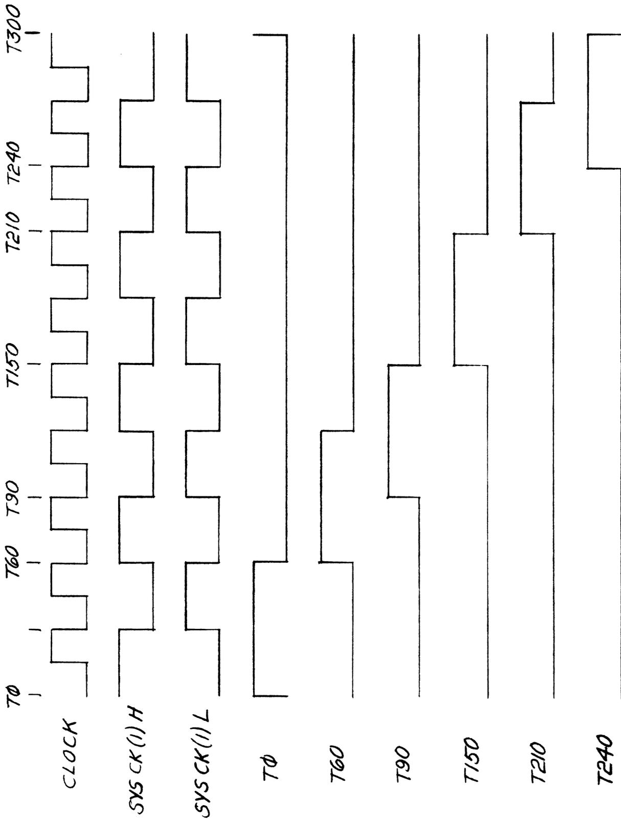
Figure 4-16 System Clock Timing Diagram
