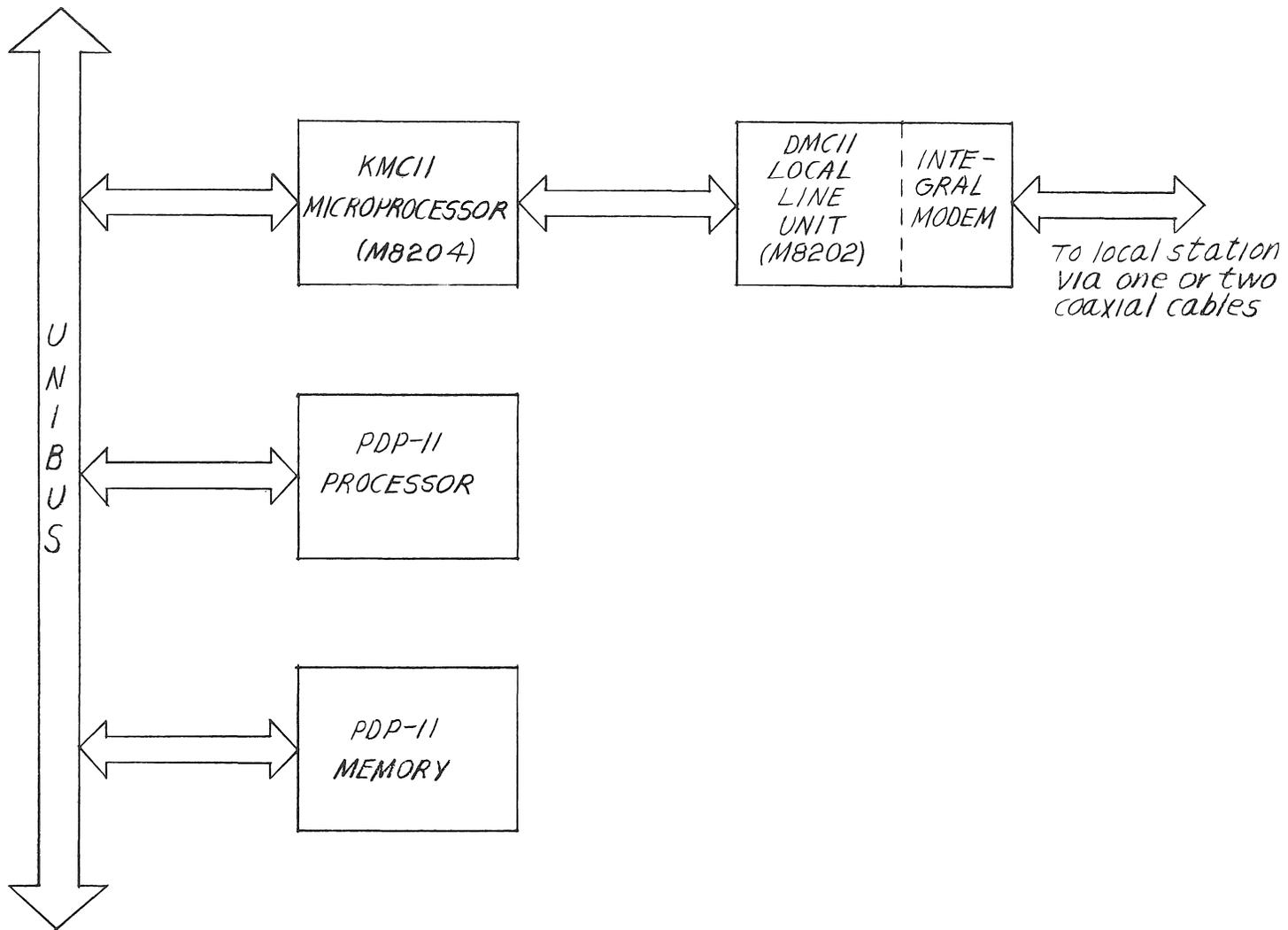
Figure 1-2 KMC11 Local Line Unit Interface
