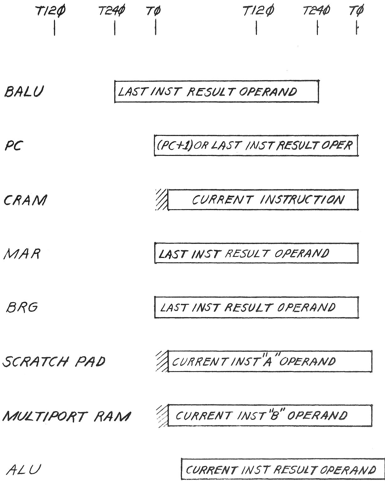
Figure 5-2 Microprocessor Register Timing
