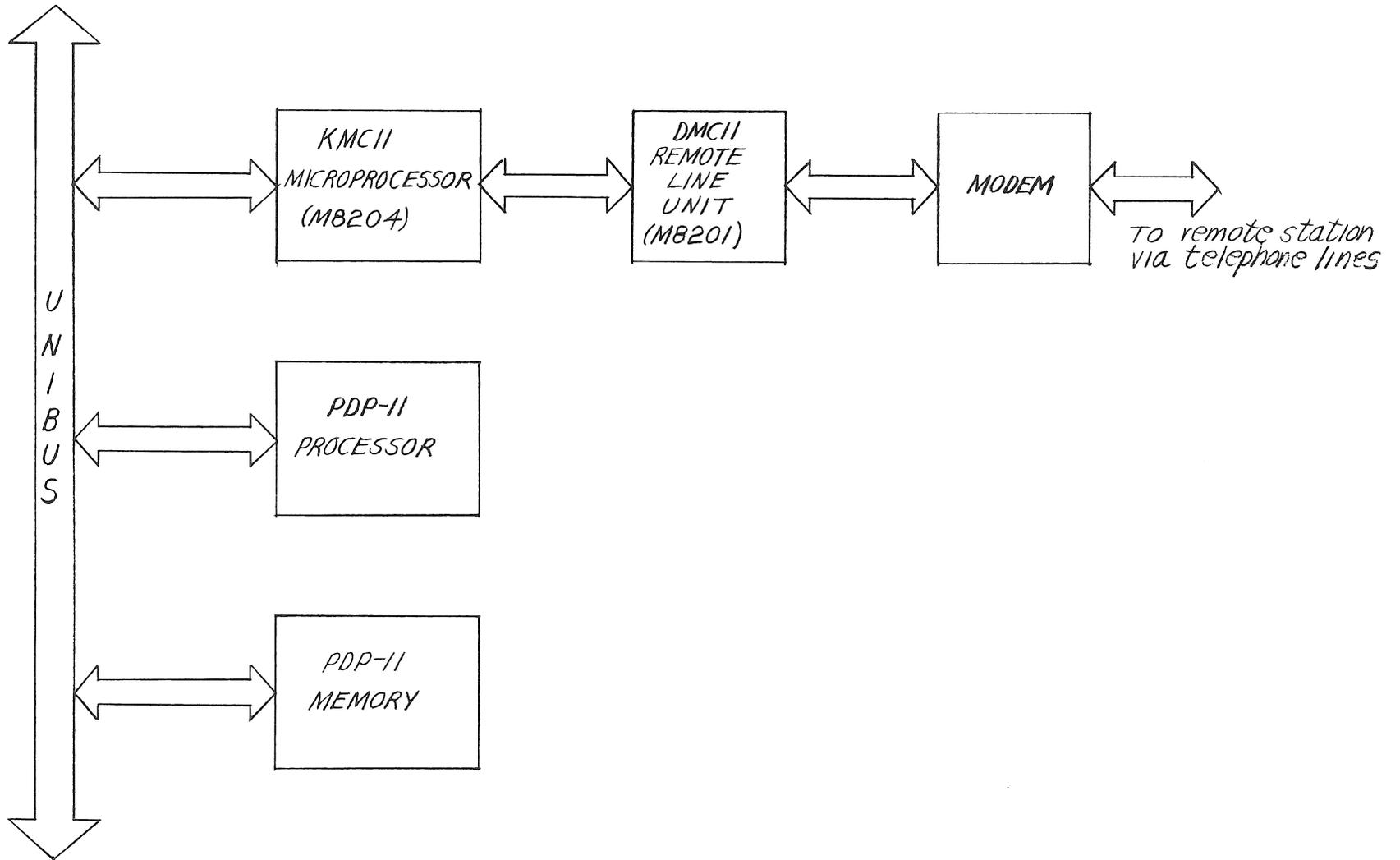
Figure 1-3 KMC11 Remote Line Unit Interface
