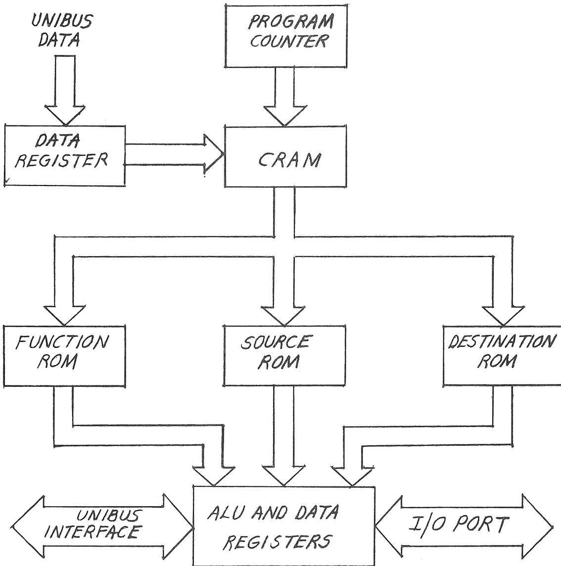
Figure 1-4 Microprocessor Simplified Block Diagram
