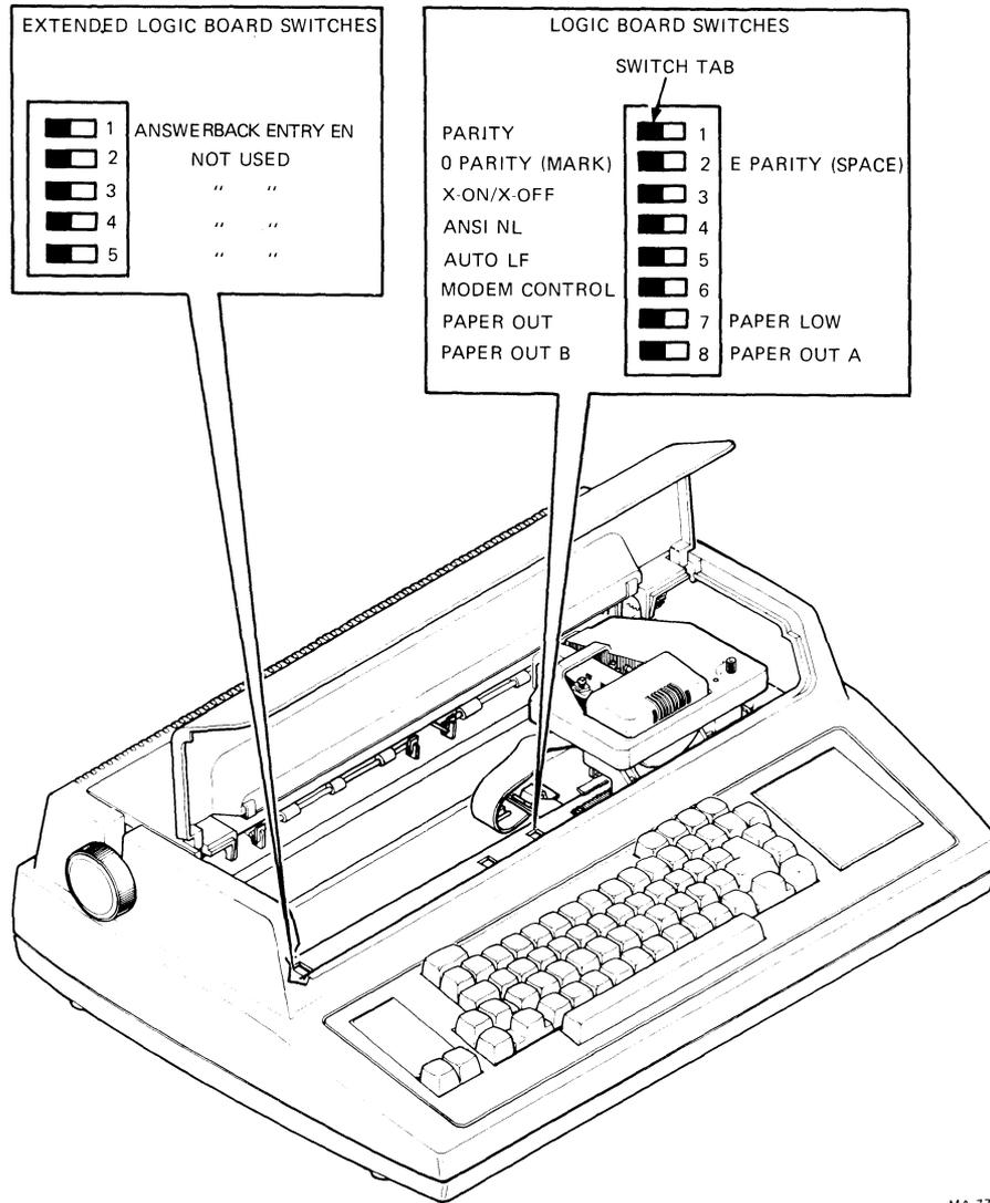
Figure 2-12 Data Communication Switches
