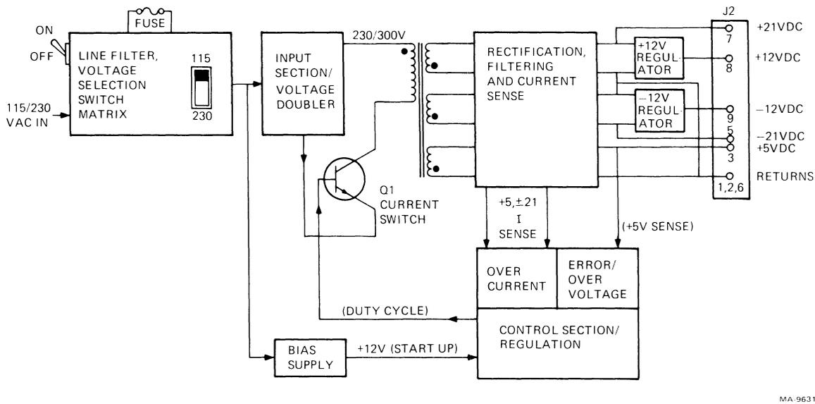
Figure 5-21 H7834 Power Supply Functional Block Diagram
