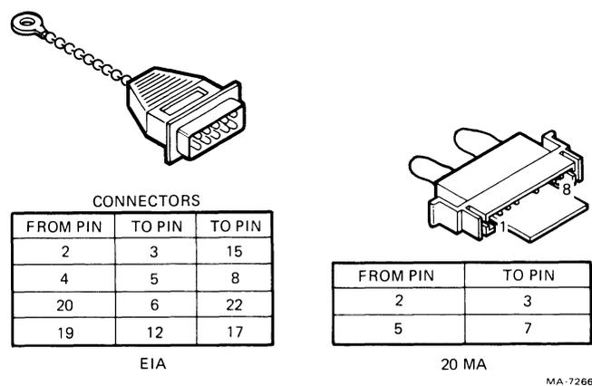
Figure 4-19 EIA and 20 mA Loopback Connectors
