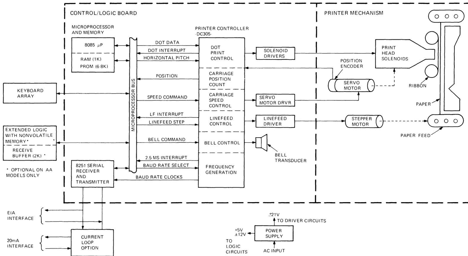
Figure 5-1 LA34 Block Diagram
