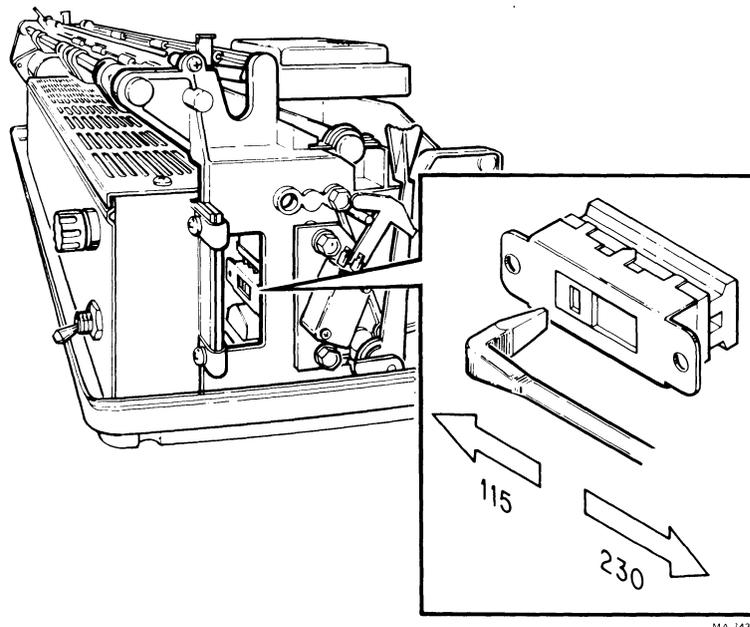
Figure 2-5 Alternate AC Voltage Selector Switch Location
