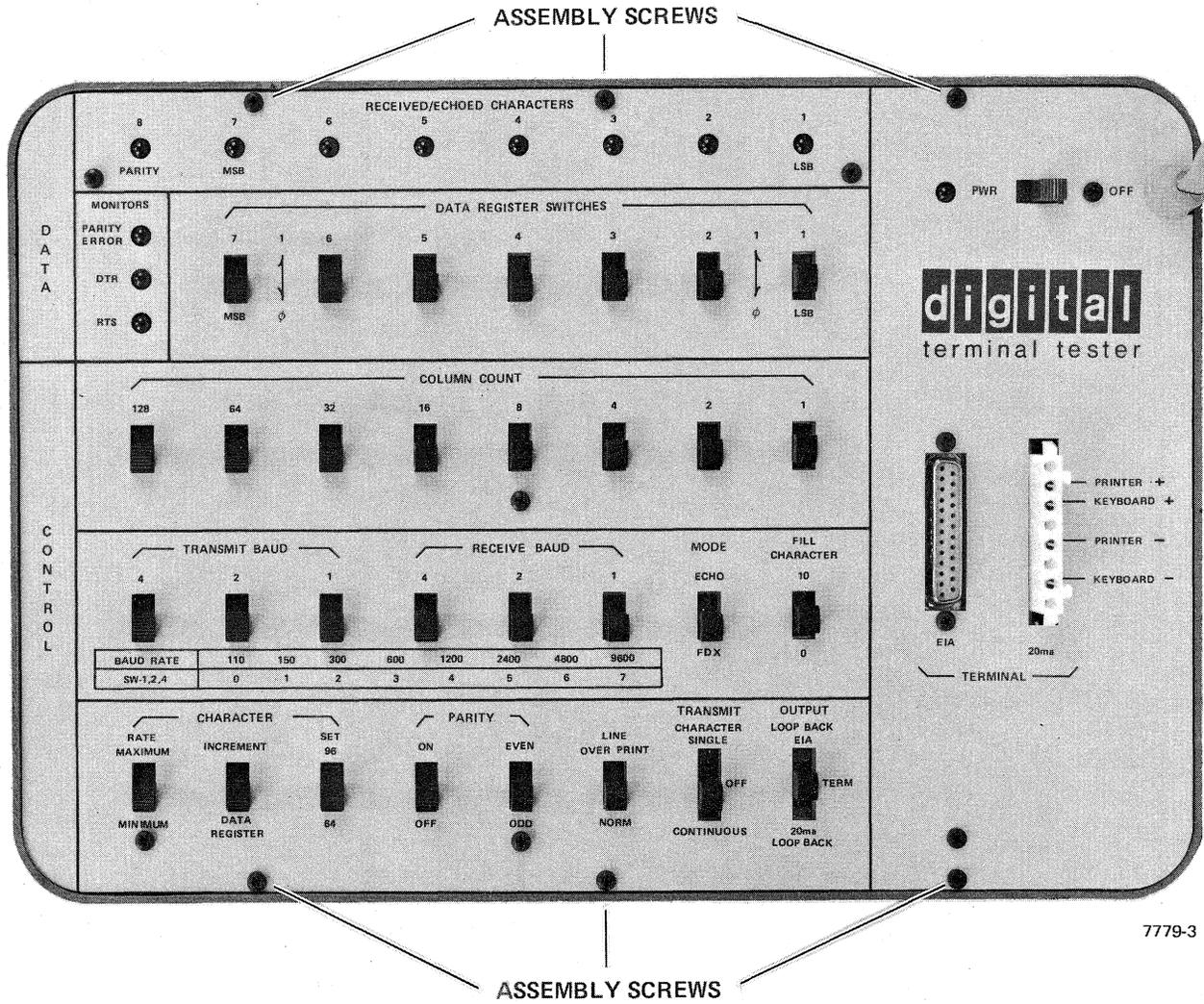
Figure 5-2 Assembly/Disassembly
