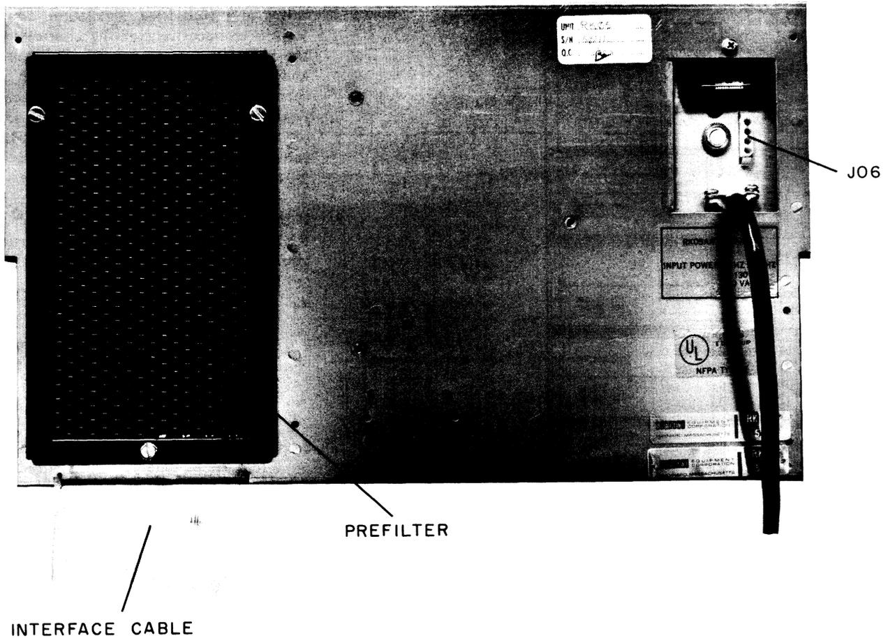
Figure 2-2 RK11C or RK11D Interface Cable Installation
