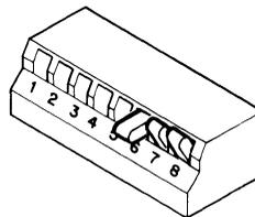
TRANSMIT AND RECEIVE SPEED FEATURES DEFAULT SET FOR 600 (RS2 AND TS2)
