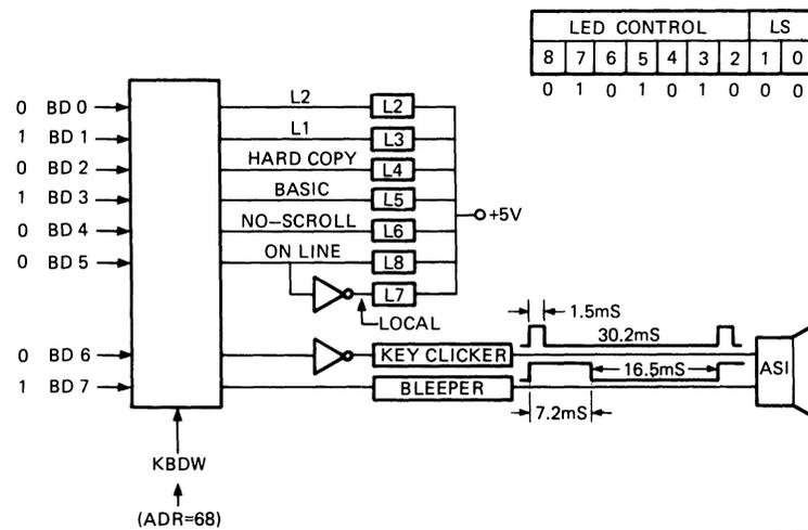
Figure 5-44 LED (Indicator) Keyclicks and Bleeper Block Diagram
