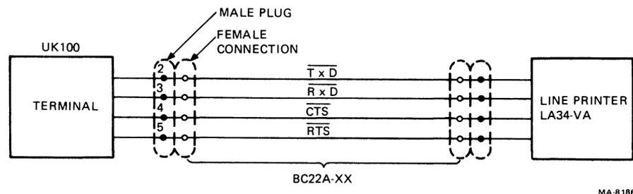
Figure 5-38 Line Printer Connected to Single Terminal
