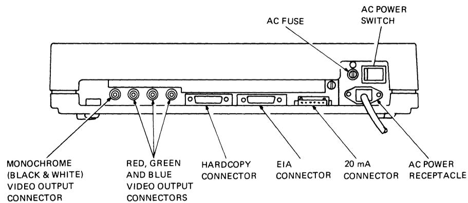
Figure 2-3 VK100 (GIGI) Terminal Switch and Cable Locations
