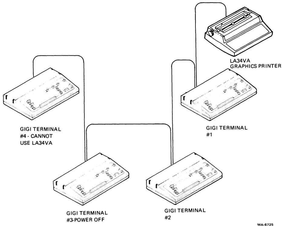
Figure 2-8 Multiterminal String with Terminal Turned Off
