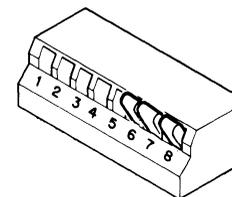
TRANSMIT AND RECEIVE SPEED FEATURES DEFAULT SET FOR 9600 (RS6 AND TS6)
