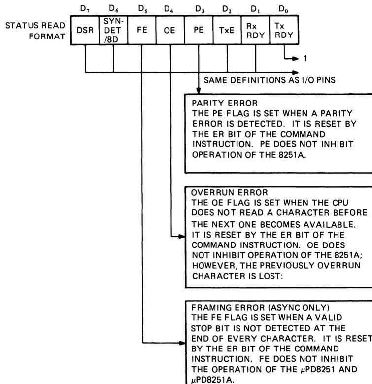
NOTE: 1 TxRDY STATUS BIT IS NOT TOTALLY EQUIVALENT TO THE TxRDY OUTPUT PIN, THE RELATIONSHIP IS AS FOLLOWS:
