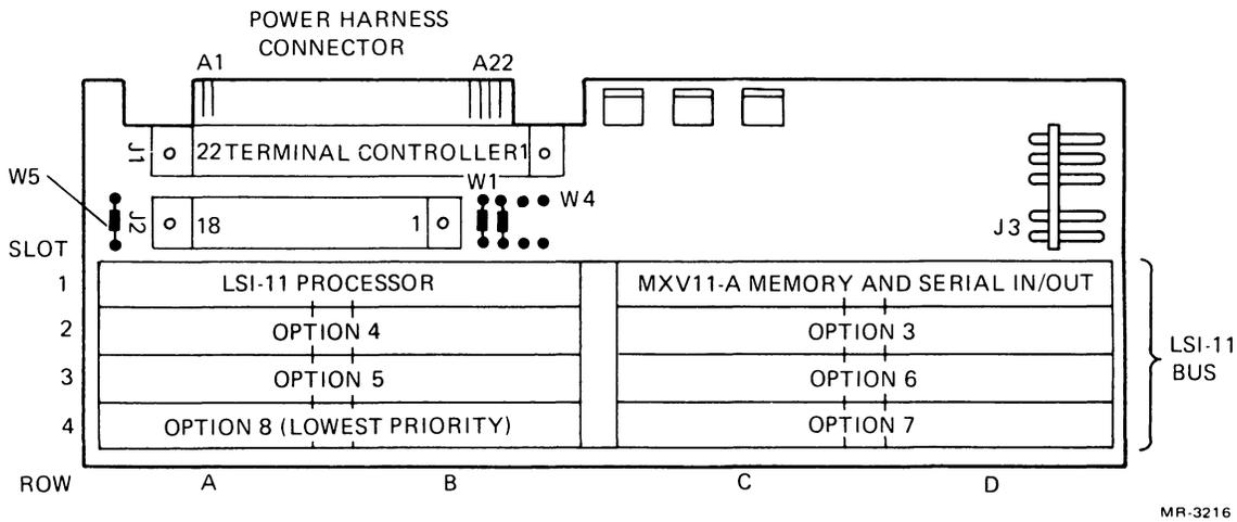
Figure 3-6 Example 2: Configuring the LSI-11 Bus
