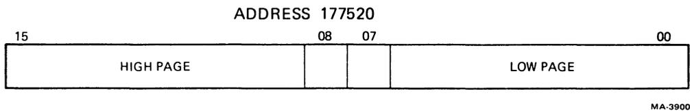
Figure 5. Page Control Register (PCR) Format
