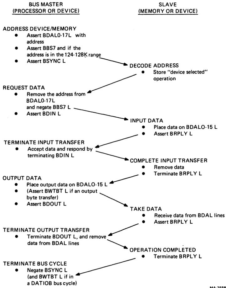
Figure 17. DATIO or DATIOB Bus Cycle
