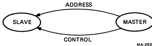
Figure 4. Master specifies type of transfer with control signals.
