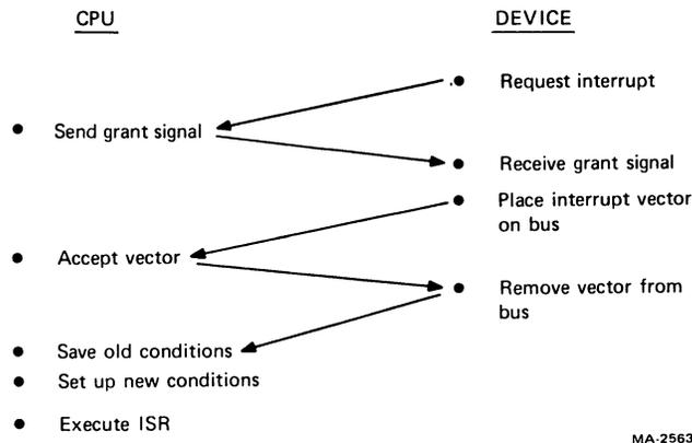
Figure 21. A Simplified Interrupt Sequence Diagram
