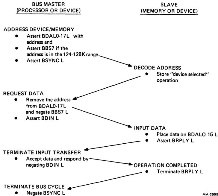
Figure 15. DATI Bus Cycle
