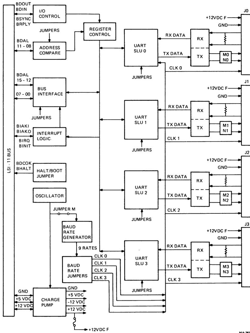
Figure 7. DLV11-J Block Diagram
