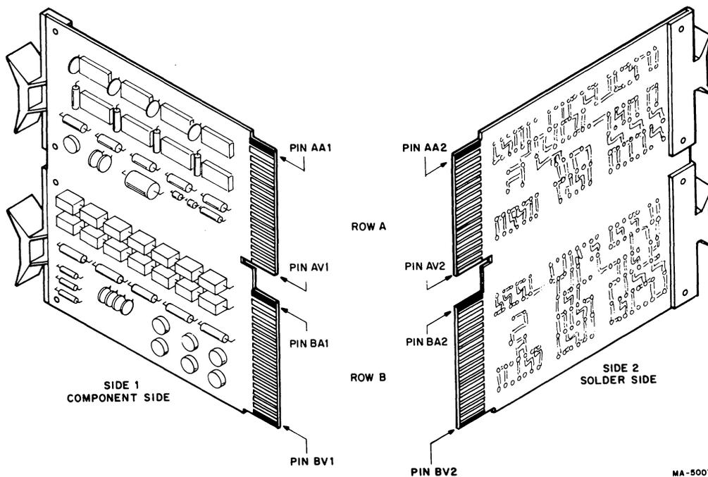
Figure 9. Double-Height Module Contact Finger Identification
