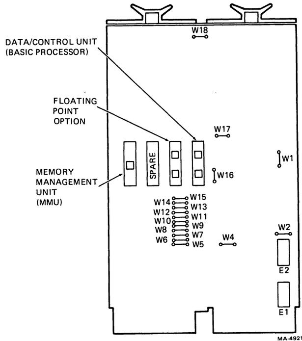
Figure 1. KDF11-AA Processor Module (M8186) with Optional Floating Point
