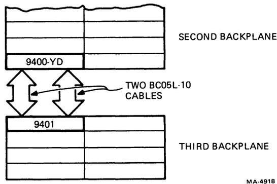
Figure 17. BCV1A Installation
