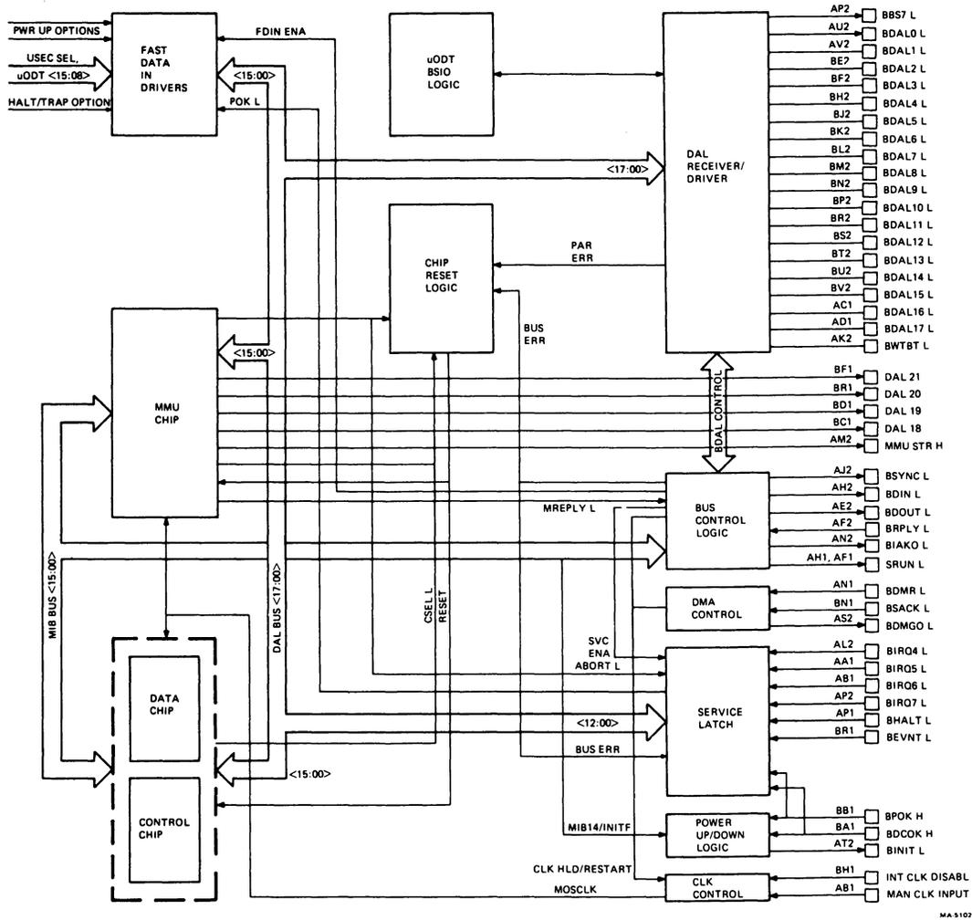
Figure 3. KDF11 Processor Block Diagram
