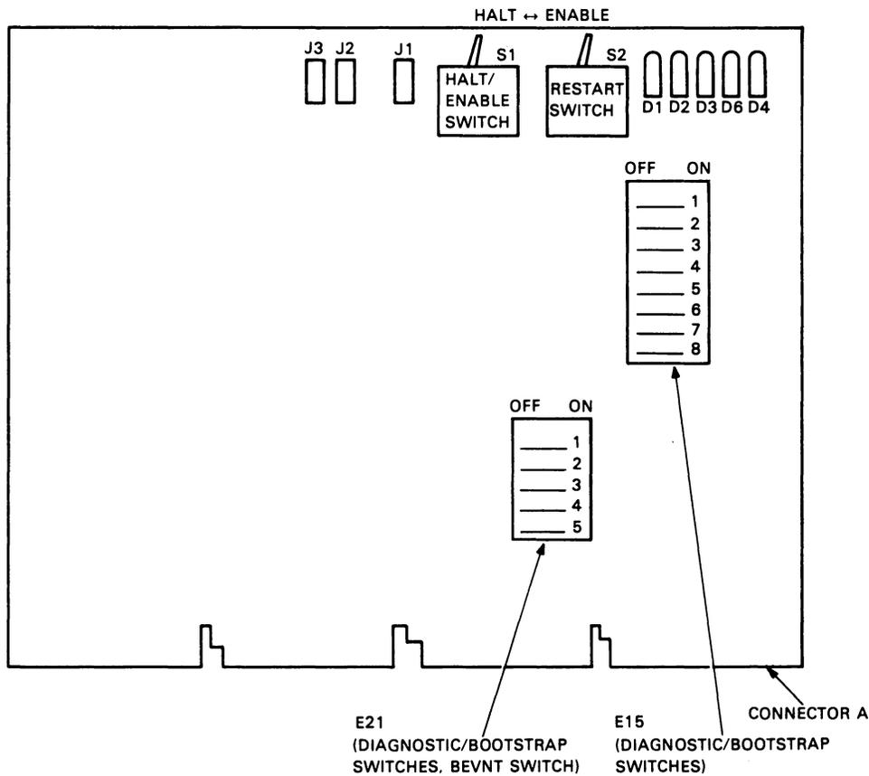
Figure 3. BDV11-AA Switches, Indicators, and Tip Jacks
