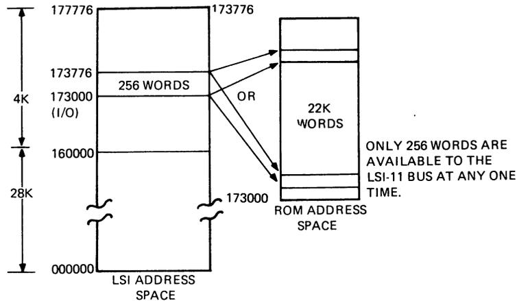
Figure 2. BDV11-AA Memory Mapping
