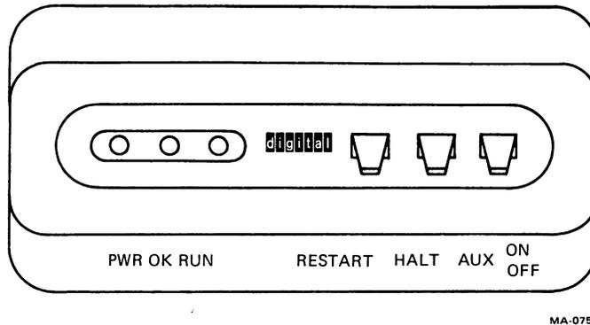
Figure 7. Front Panel Switches and Indicators
