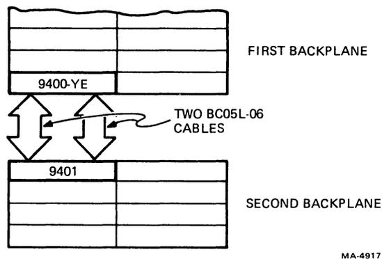
Figure 15. BCV1B Installation
