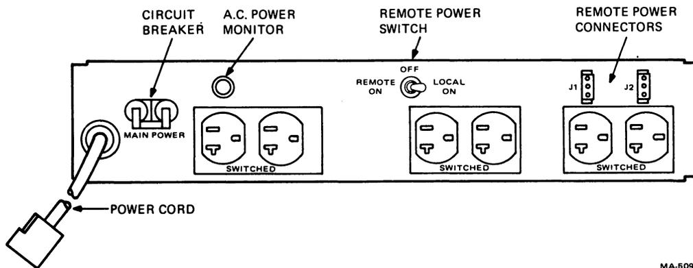
Figure 5. Power Controller (Rear View)
