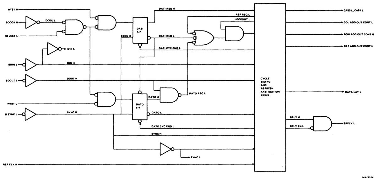
Figure 7. Timing and Control Logic
