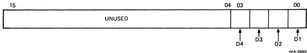
Figure 7. Display Register Format
