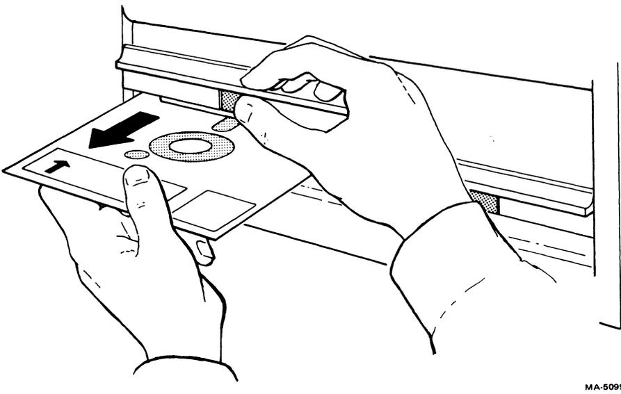
Figure 2. Removing the Diskette
